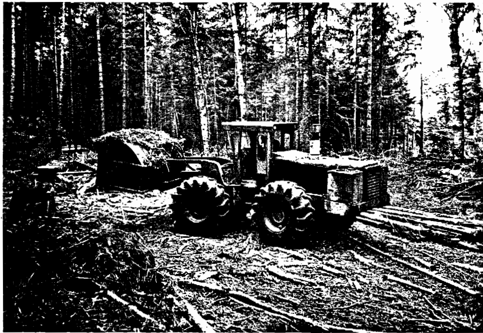
Figure 8. Hydro-Ax chain flail delimeter.
