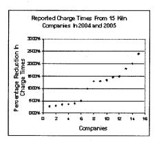
When we looked at, from one particular company that gave us more complete data, some of the three month baseline data (before installation) from 2004 with the same period of time post-installation the trend was generally down but in a few cases in some kilns it went up and tended to reduce the system average when we ran it through our statistical software package.
