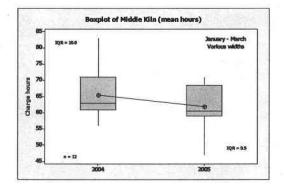
The Middle kiln plot shows that the mean drying time improvement trend continues. The gains on process variation, seen with the other kilns, aren't as great here, as shown with an interquartile drop of 10 to 9.5. This is probably due to the as yet, undiscovered variation. However, the mean drying time reduction is still a robust 5.47%.
