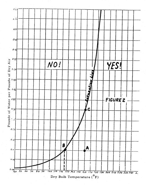
additional moisture vapor is added condensation will take place to maintain the moisture content at the saturation level.
