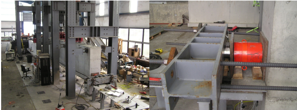
Fig. 3.50 – Post tensioned bent cap installation: overall view (left) actuator and reaction beam (right).
