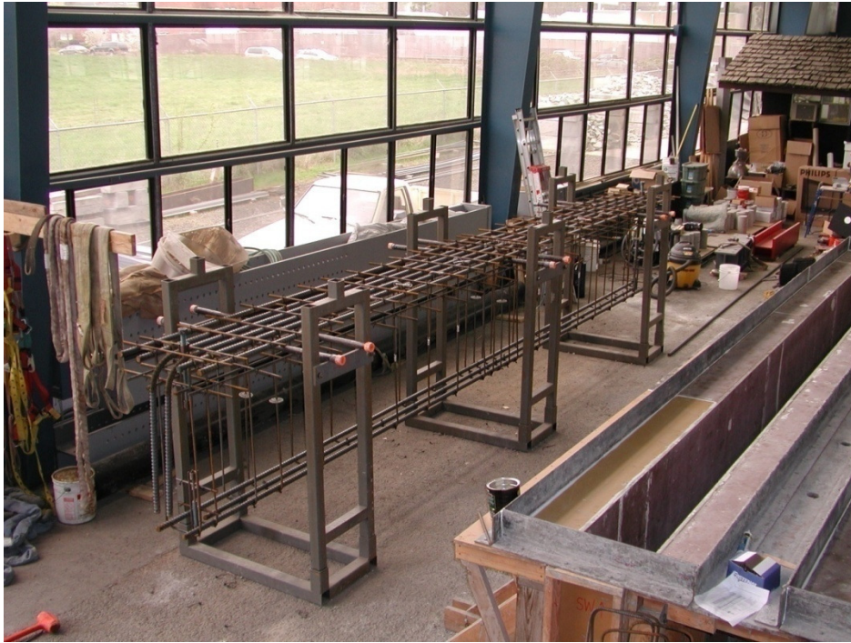
Fig. 3.33 – Assembly of completed reinforcing cage adjacent to formwork (IT specimen shown).
