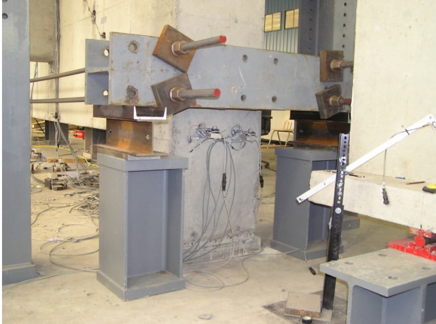
Fig. 3.51 – Post tensioned bent cap installation: adjacent reaction beam.
