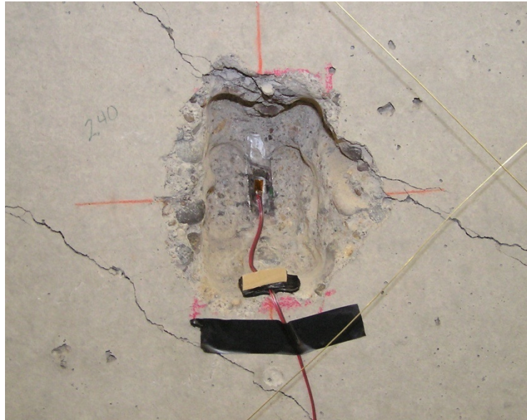
Fig. 4.8 – Exposure of integrally cast stirrup leg to replace failed strain gage
