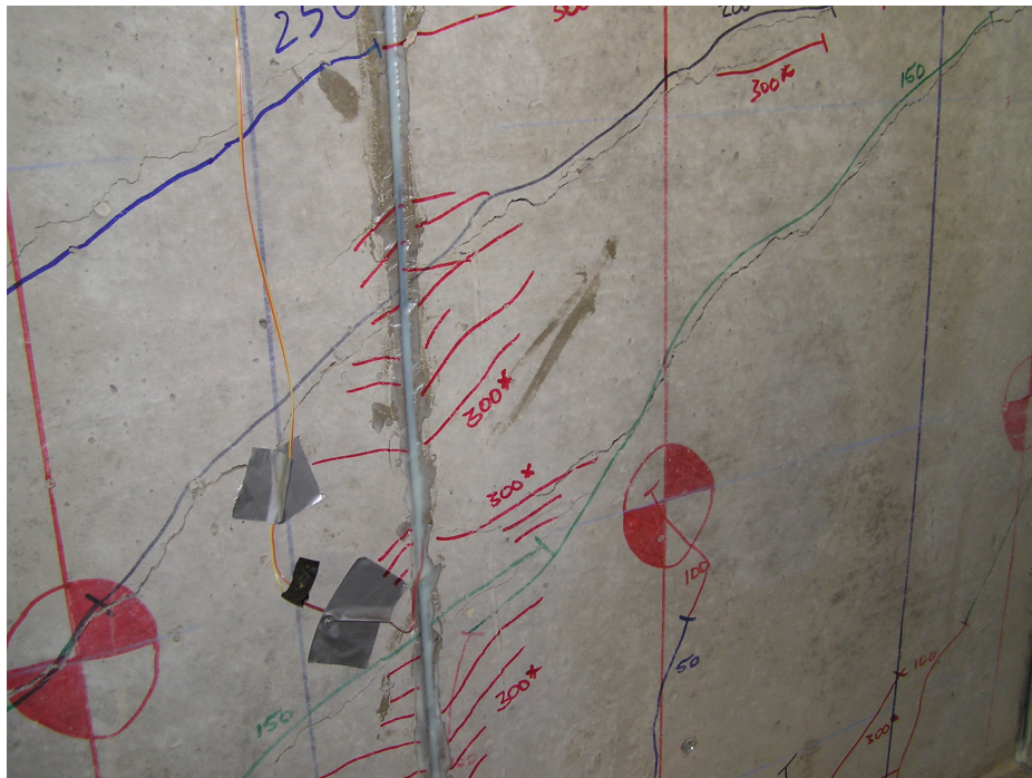
Fig. 5.27 – B.IT.NC.NS restraint of cracks under load
