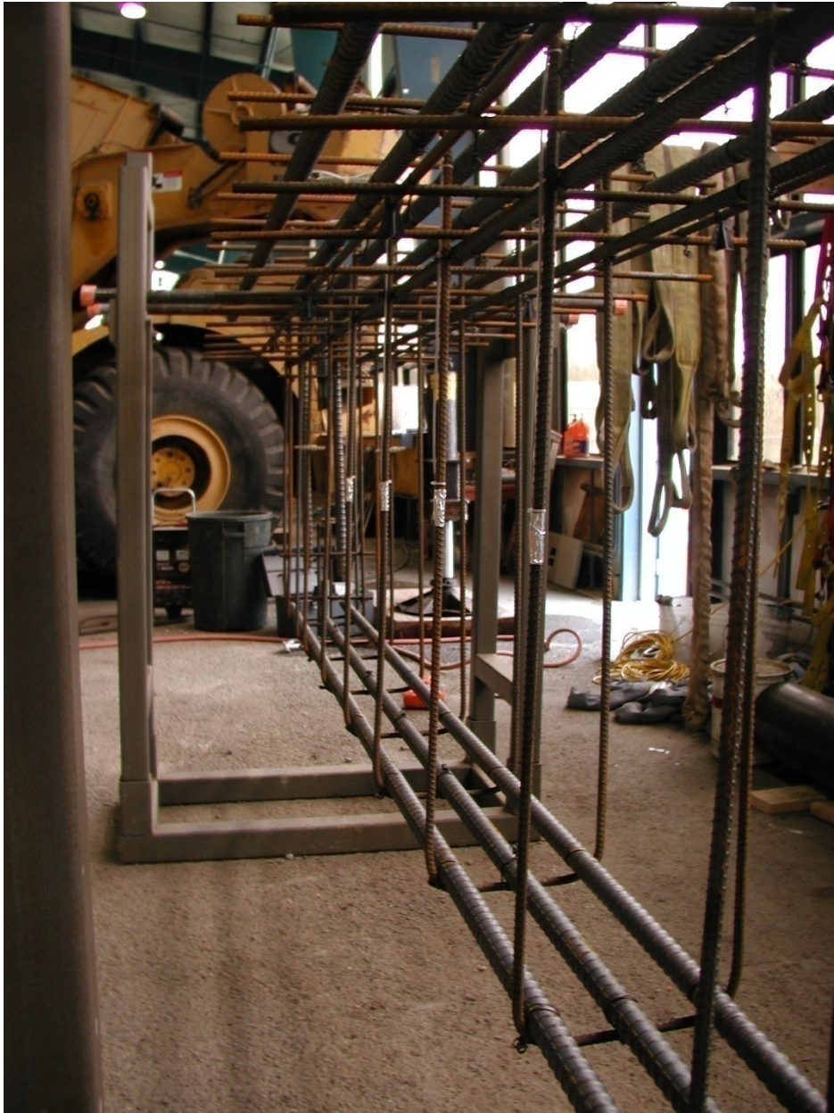
Fig. 3.32 – Typical strain gage locations along stirrups.
