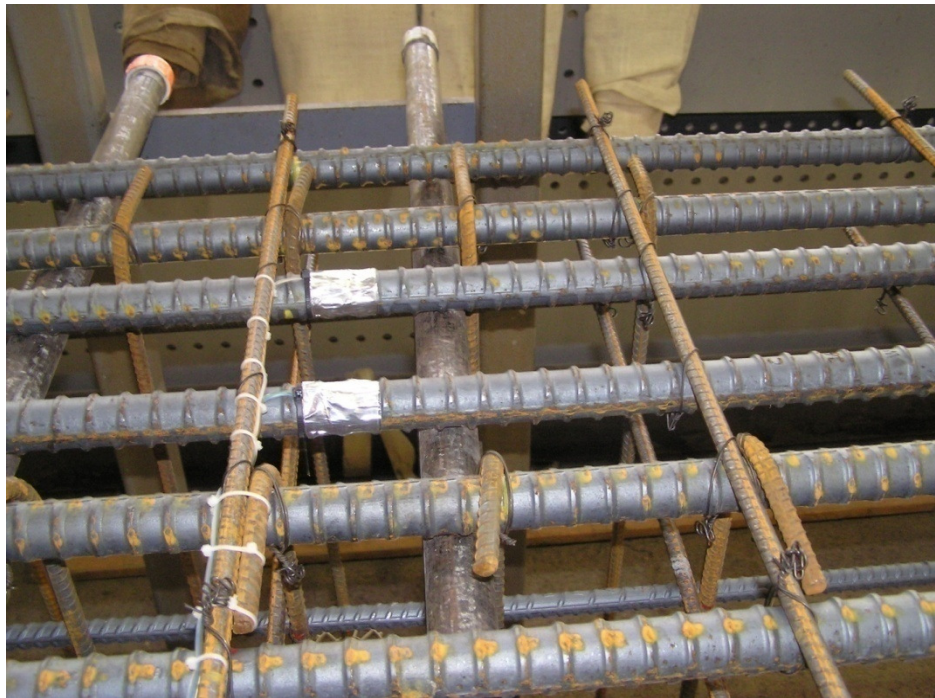
Fig. 3.31 – Typical strain gage locations along flexural steel.
