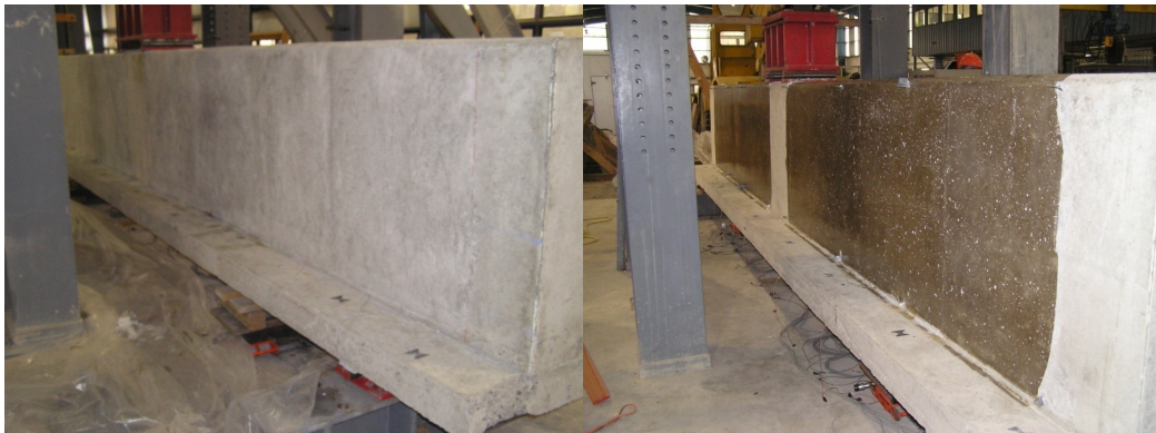
Fig. 3.43 – CFRP installation: ground surface (left) and primer application (right).
