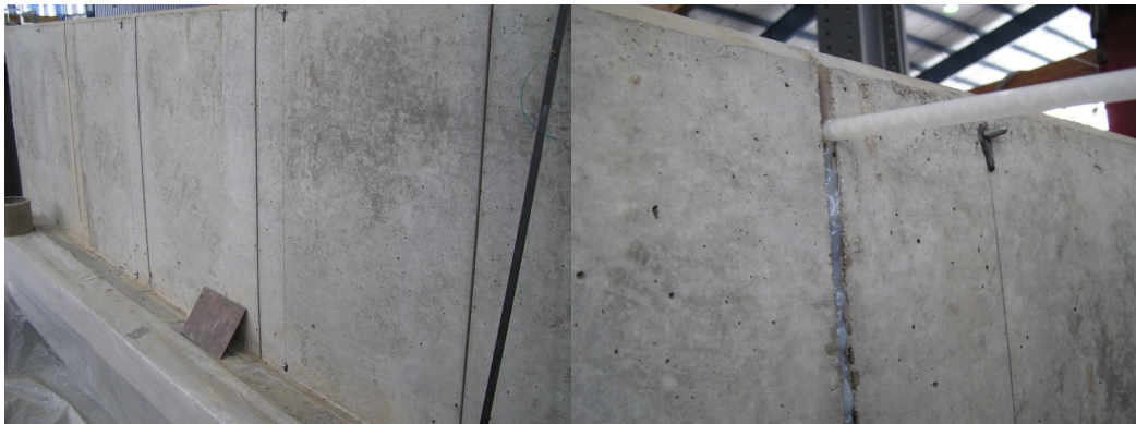
Fig. 3.45 – NSM installation: cut grooves (left) and initial epoxy application (right).
