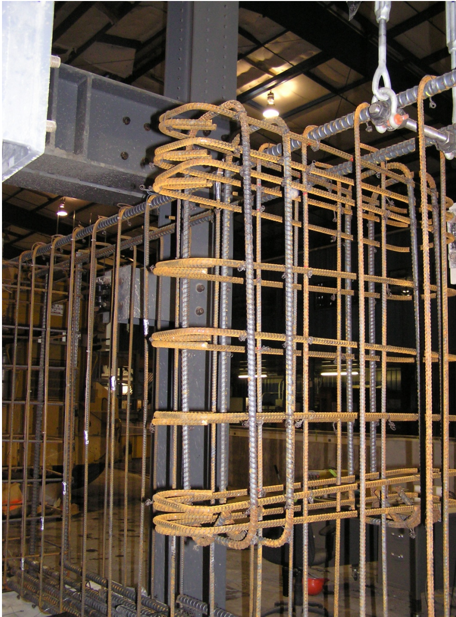
Fig. 3.36 – Typical bent cap stub girder assembly.
