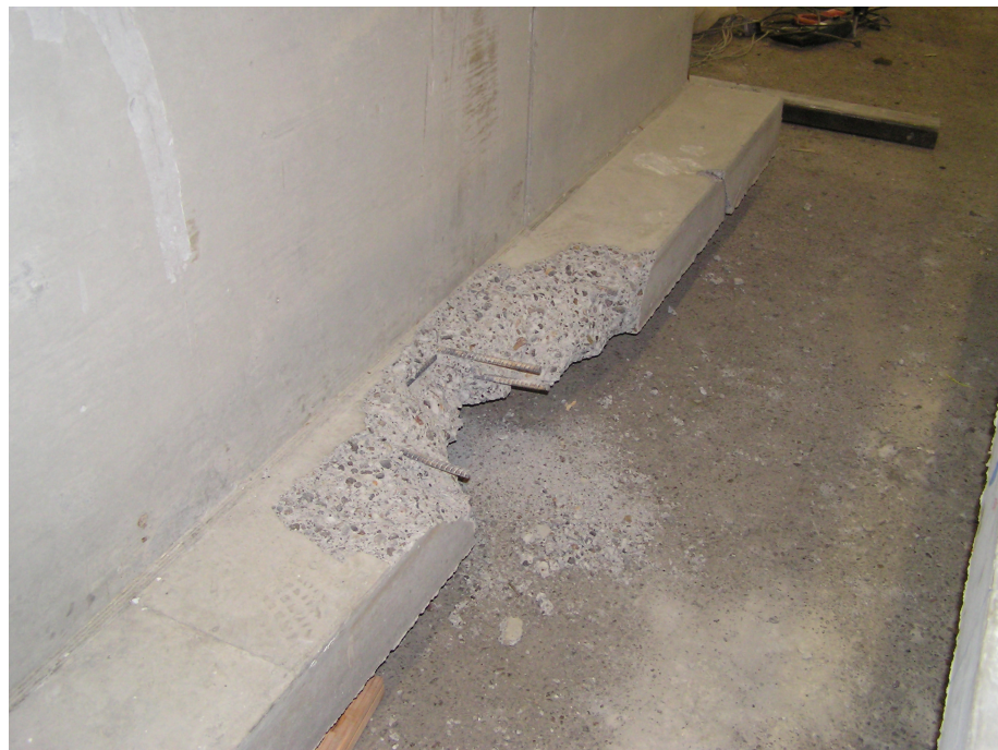
Fig. 4.47 – B.IT.C.IS flange damage: a) top of flange and b) side of flange
