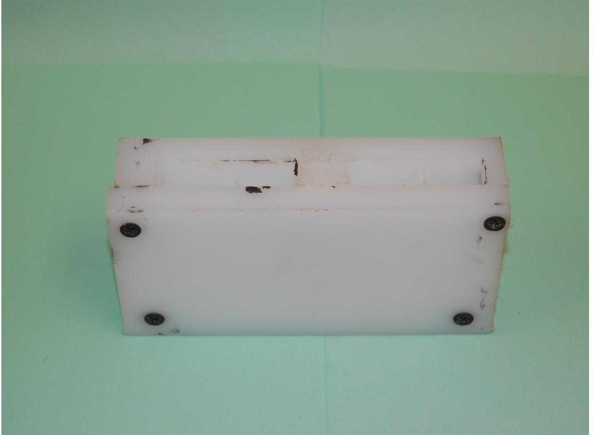
Figure 2.3: Aligned Macro-magnetic Composite Mold
