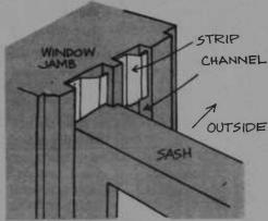
Installation (lower sash)—Install strips full width of sash on bottom of lower sash bottom rail and top of upper sash top rail.
