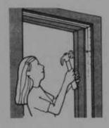
Interlocking Metal Channels—Difficult to install (alignment is critical). Visible when installed. Durable but subject to damage. Excellent seal.
