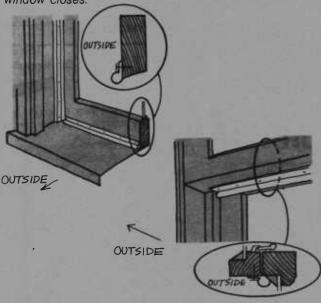
Pliable Gaskets—Foam rubber attached with adhesive backing or flexible vinyl, rubber or felt attached with brads or staples. Easy to install. Out of sight. Breaks down and wears rather quickly. Not as effective a sealer as metal strips or rolled vinyl. Never use where friction occurs.
