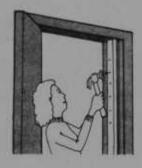
Foam Rubber with Wood Backing—Easy to install. Visible when installed. Not very durable.
