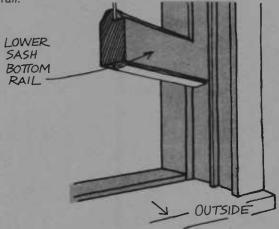
Installation (upper sash)—Attach a strip full width of window to upper sash bottom rail. Countersink nails slightly so they do not catch on lower sash top rail.
