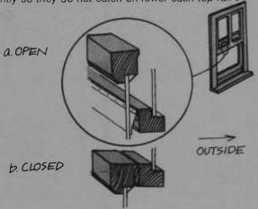
Rolled Vinyl or Rigid Strip Gasket (with or without metal backing)—Visible when installed. Easy to install. Durable. Installation—Nail vinyl strips on double-hung windows as shown. A sliding window is much the same and can be treated as a double-hung window turned on its side. Casement and tilting windows should be weather stripped with vinyl nailed to window casing so roll is compressed as window closes.
