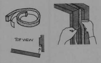
Rolled Vinyl with Aluminum Channel Backing—Easy to install. Visible when installed. Durable.
