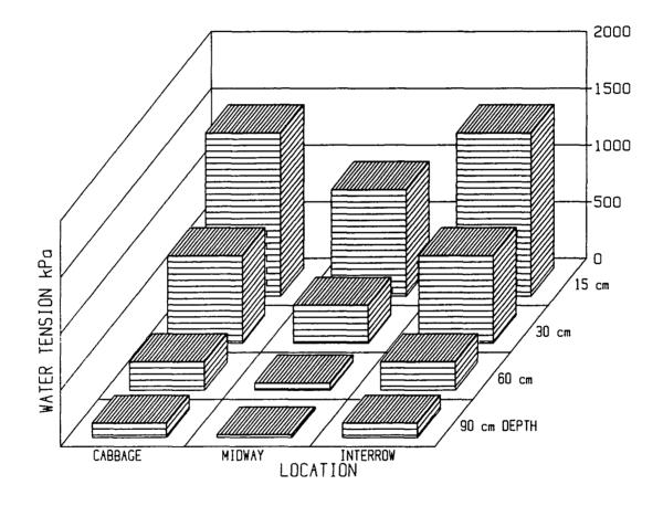
Figure 3.4. Seasonal average water tension (kPa) as measured by gypsum blocks in the double density cabbage treatment.
