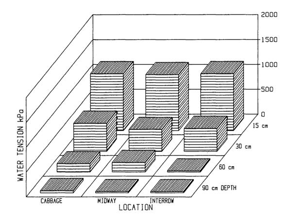
Figure 3.6. Seasonal average water tension (kPa) as measured by gypsum blocks in the mowed grass treatment.
