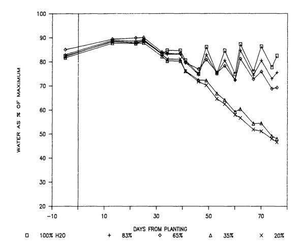
Figure 3.8. The effect of water applied on the amount of water in the 105 cm soil profile as measured over the season by the neutron meter. Average of both interrow treatments. Water is expressed as a percent of the maximum measurement.
