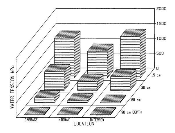
Figure 3.5. Seasonal average water tension (kPa) as measured by gypsum blocks in the unsuppressed grass treatment.
