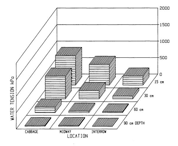
Figure 3.3. Seasonal average water tension (kPa) as measured by gypsum blocks in the low density cabbage treatment.
