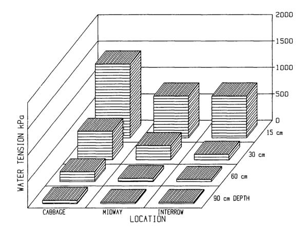
Figure 3.7. Seasonal average water tension (kPa) as measured by gypsum blocks in the chemically suppressed grass treatment.
