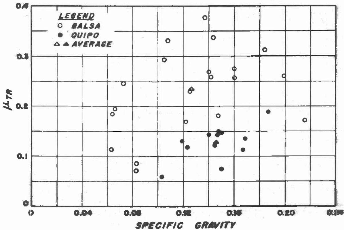
Figure 14.--Poisson's ratio ( $\mu_{TR}$ ) plotted against specific gravity for balsa and quipo.
