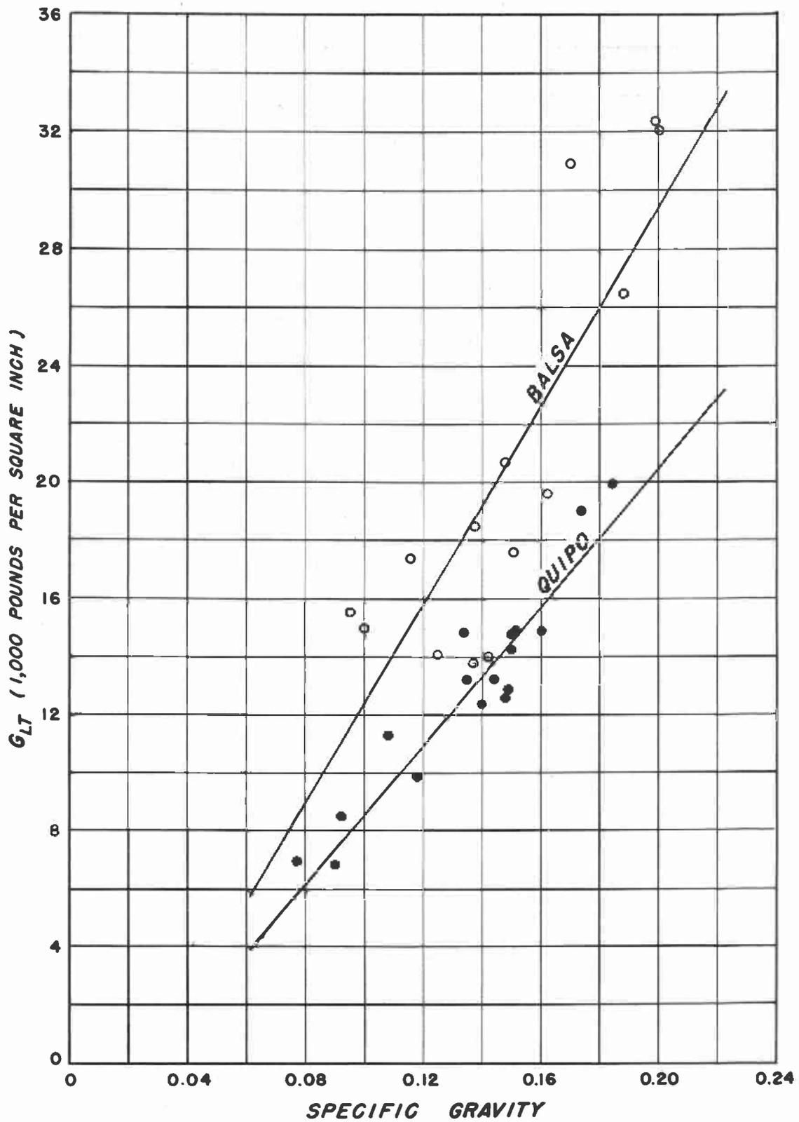
Figure 17.--Relation of modulus of rigidity ( $G_{LT}$ ) to specific gravity for balsa and quipo.
