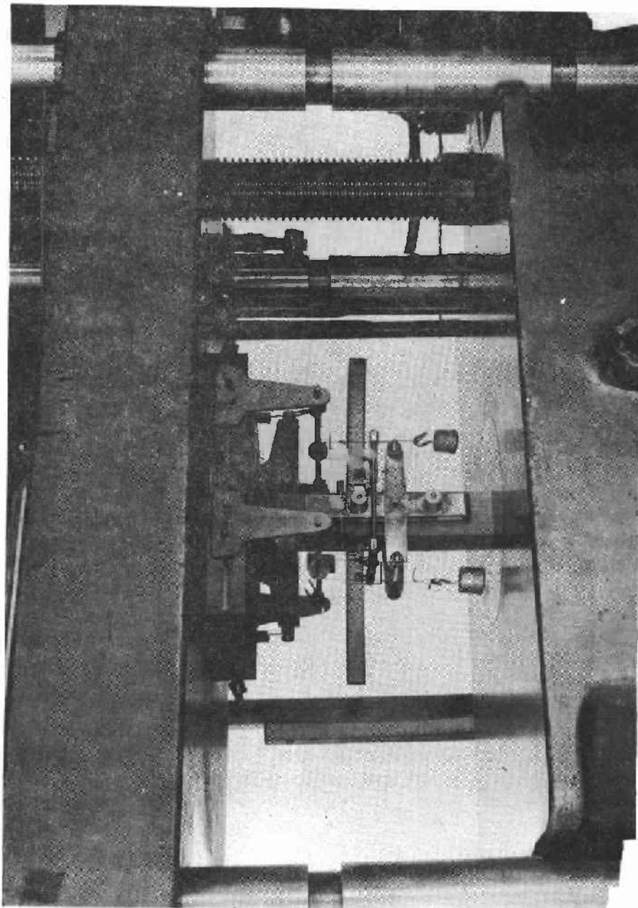
Figure 3.--Method of measuring Young's moduli and Poisson's ratios, showing axial and lateral extensometers, and scales for measuring deformation.
