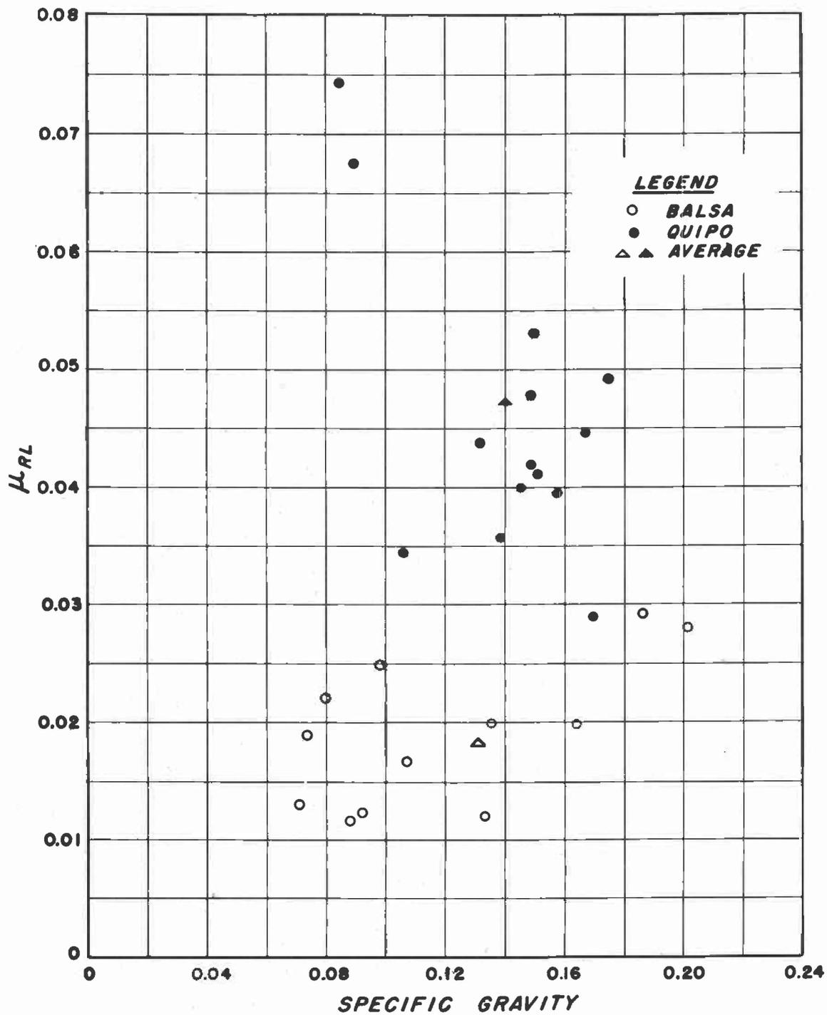
Figure 13.--Poisson's ratio ( $\mu_{RL}$ ) plotted against specific gravity for balsa and quipto.
