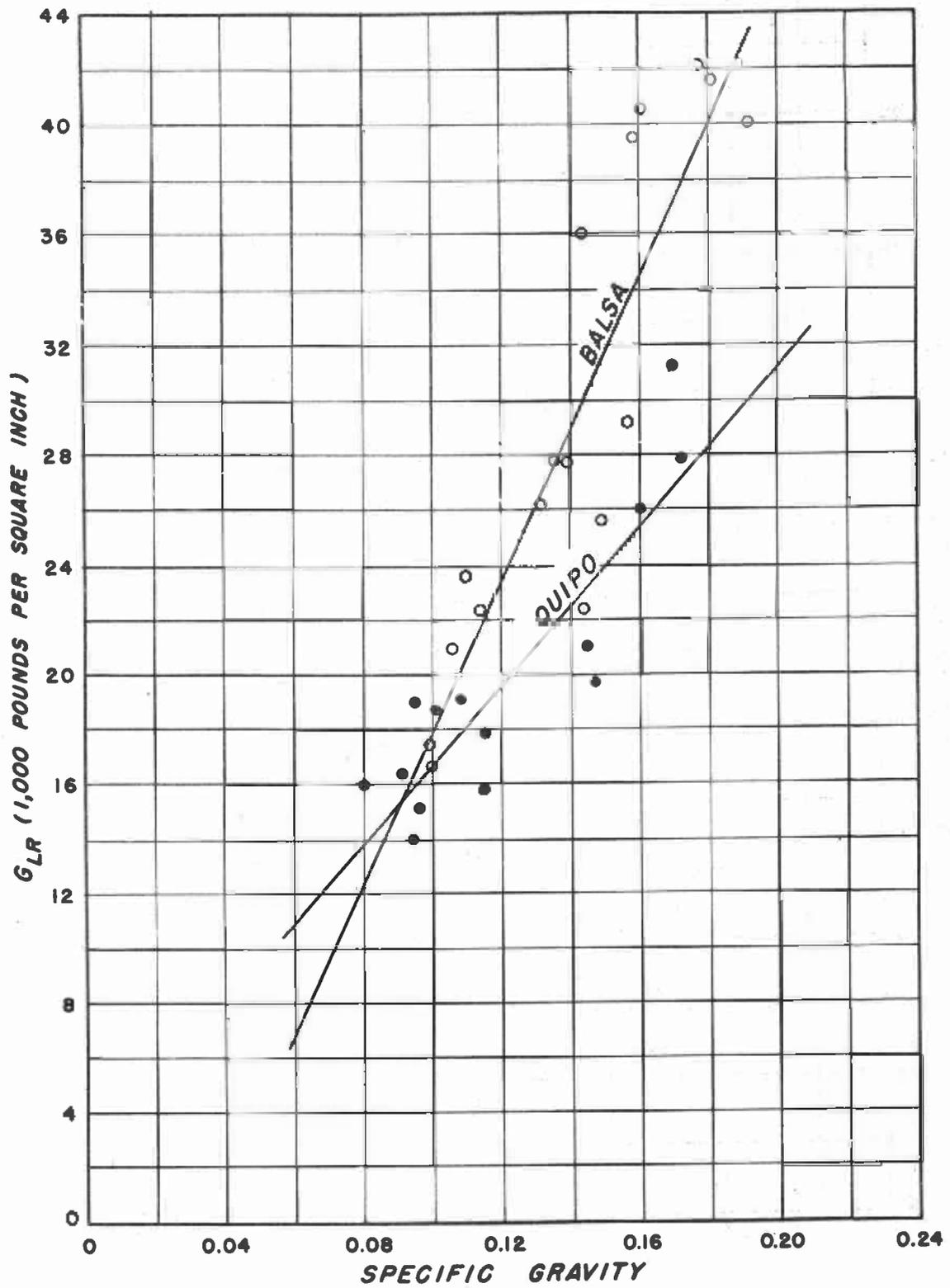
Figure 16.--Relation of modulus of rigidity ( $G_{LR}$ ) to specific gravity for balsa and quipo.
