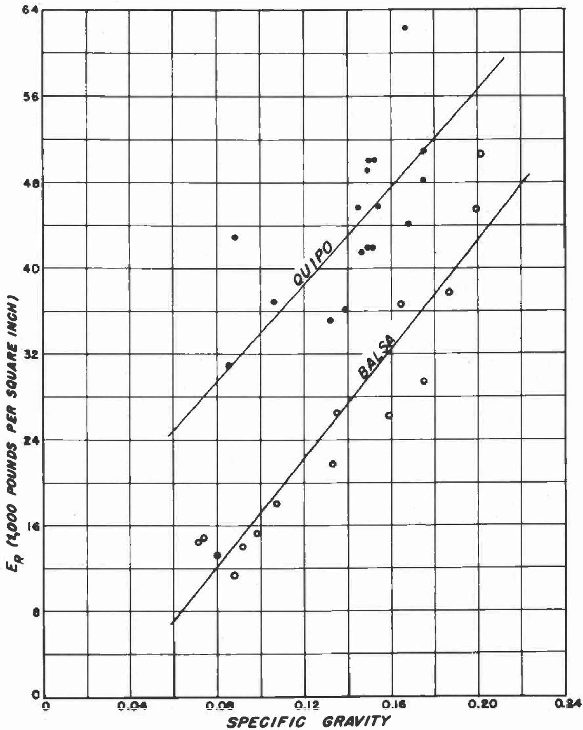
Figure 8.--Relation of modulus of elasticity in the radial direction ( $E_R$ ) with specific gravity for balsa and quipo.
