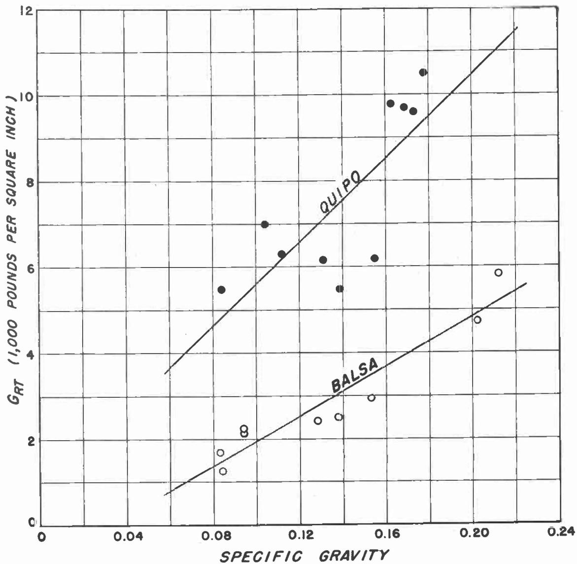
Figure 18.--Relation of modulus of rigidity ( $G_{RT}$ ) to specific gravity for balsa and quipo.
