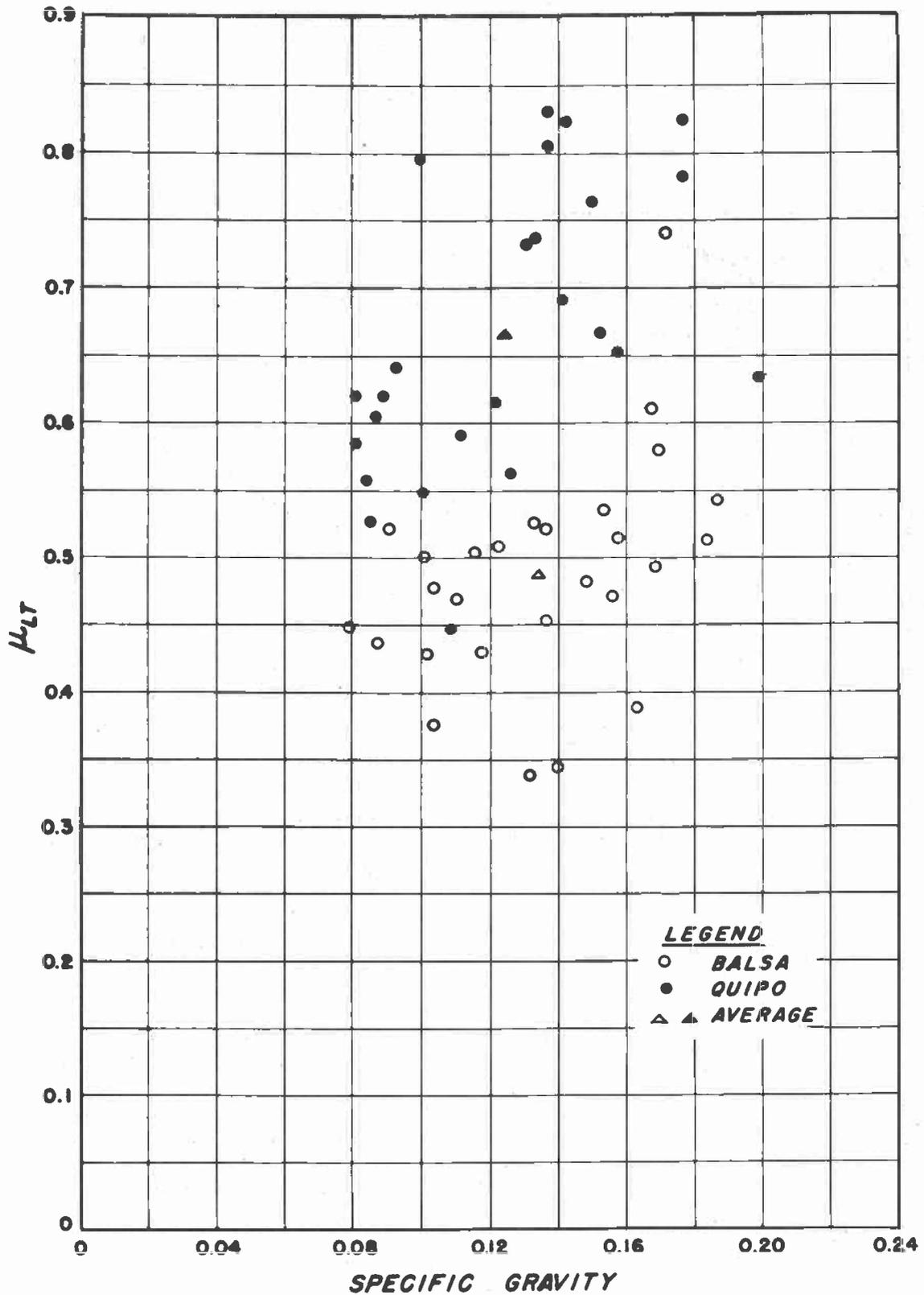
Figure 10.--Poisson's ratio ( $\mu_{LT}$ ) plotted against specific gravity for balsa and quipto.
