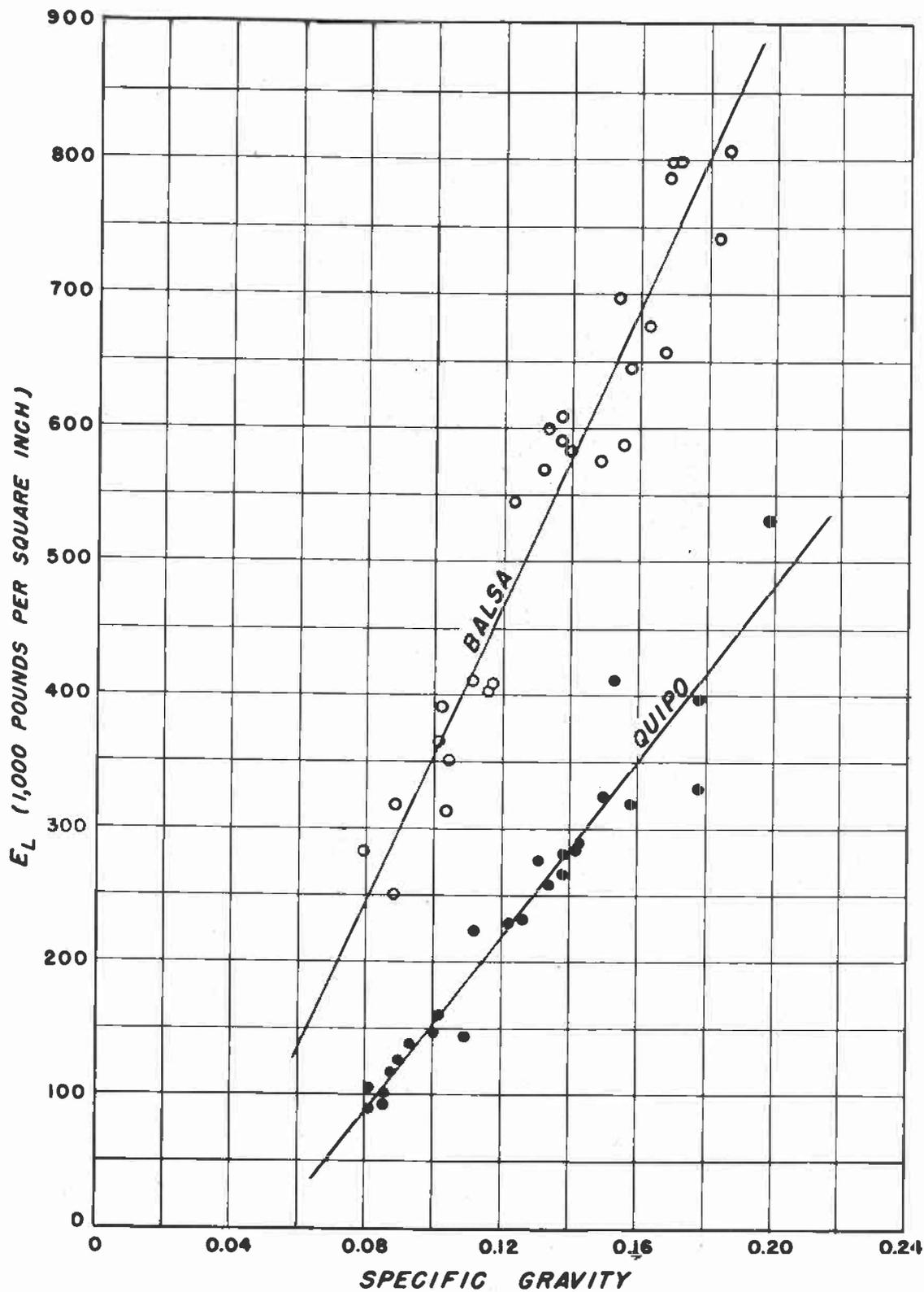
Figure 7.--Relation of modulus of elasticity in the longitudinal direction ( $E_L$ ) with specific gravity for balsa and quipo.
