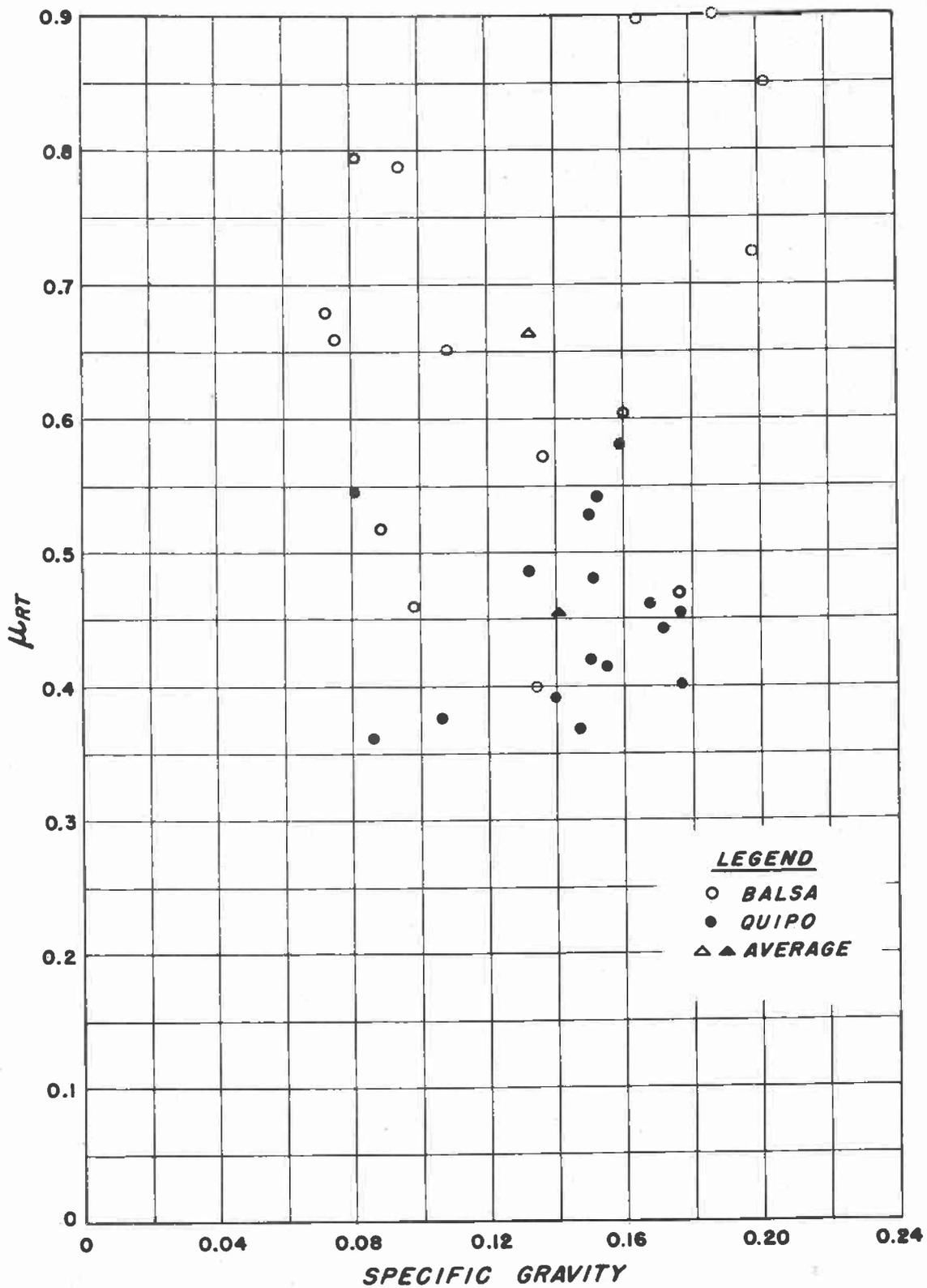
Figure 12.--Poisson's ratio ( $\mu_{RT}$ ) plotted against specific gravity for balsa and quipto.
