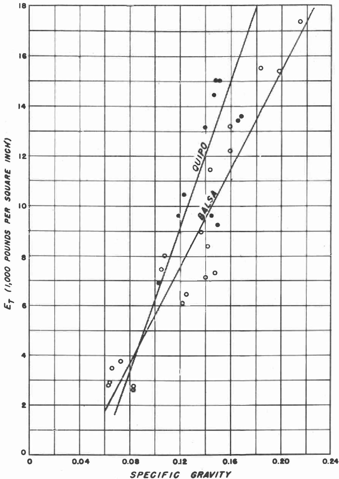
Figure 9.--Relation of modulus of elasticity in the tangential direction ( $E_T$ ) with specific gravity for balsa and quipo.
