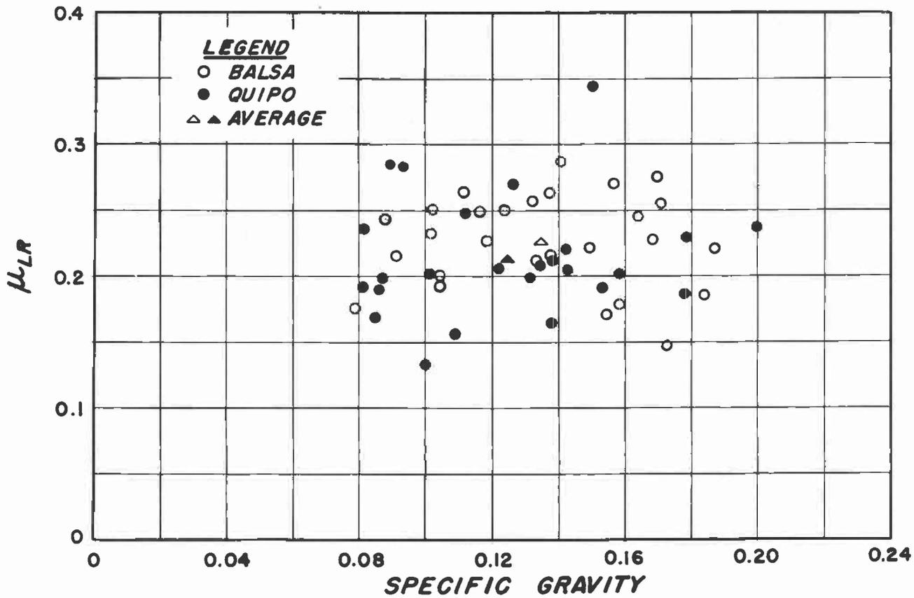
Figure 11.--Poisson's ratio ( $\mu_{LR}$ ) plotted against specific gravity for balsa and quiipo.
