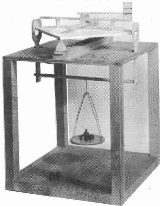
Figure 6.--Special plate shear apparatus used for
