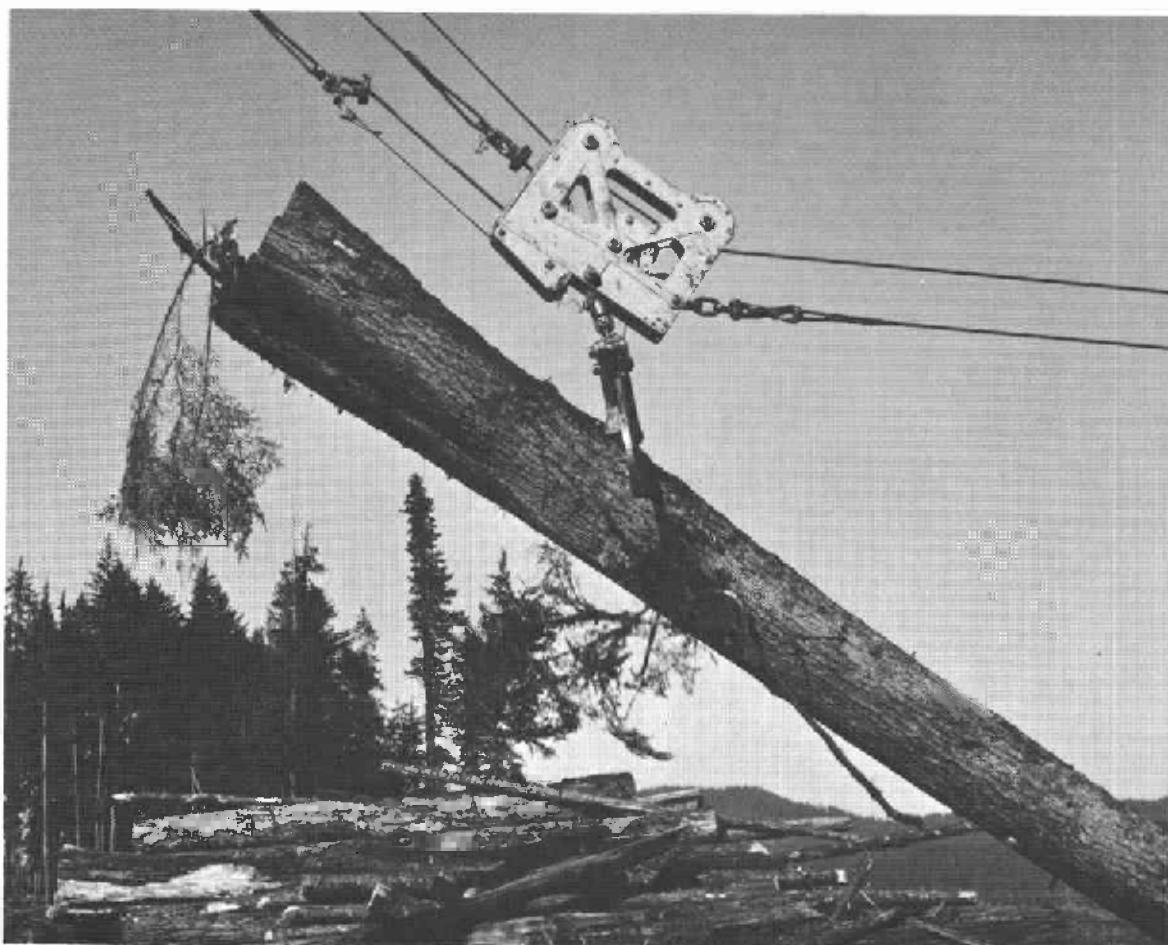
A combination grapple-carriage makes for efficient skyline logging.
