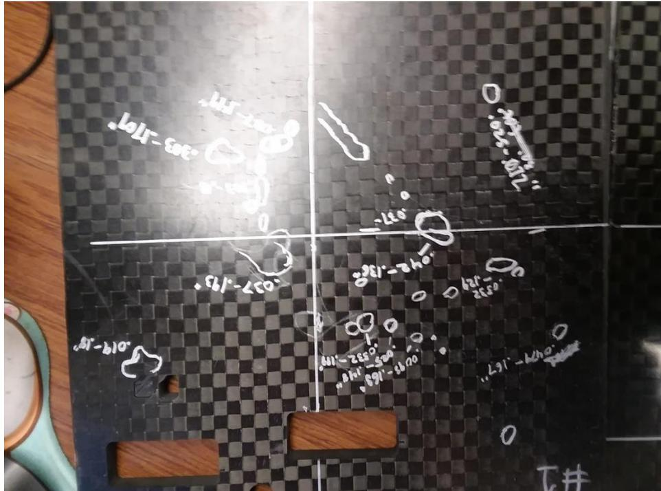
Fi 17. CFRP Panel (With defects marked out after scan).
