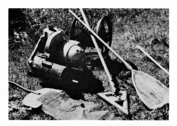
Figure 4. Direct current generator used in electrofishing accessible stream area.
