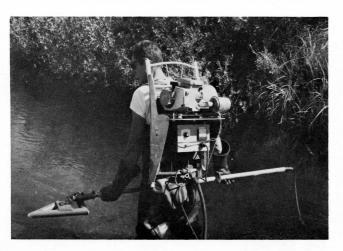
Figure 5. Backpack electrofishing unit for use in inaccessible stream areas.
