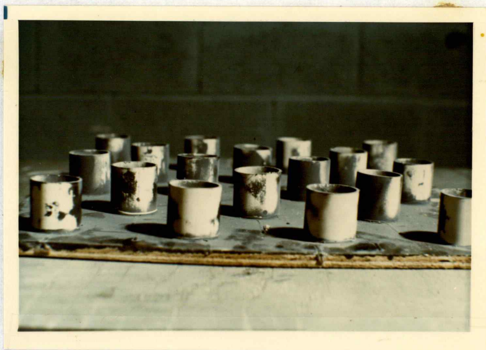
Figure 37. Photograph showing areas where black paint has been worn off of white tube material, suggesting areas where tube erosion might be of concern.
