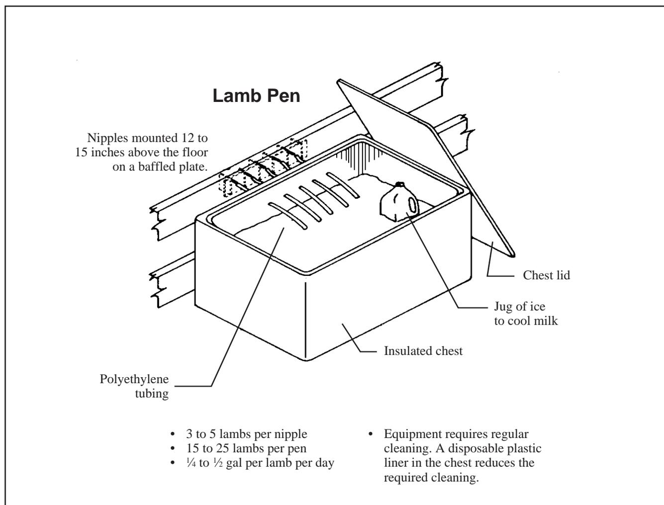
Figure 2.—An example of a milk reservoir setup.
