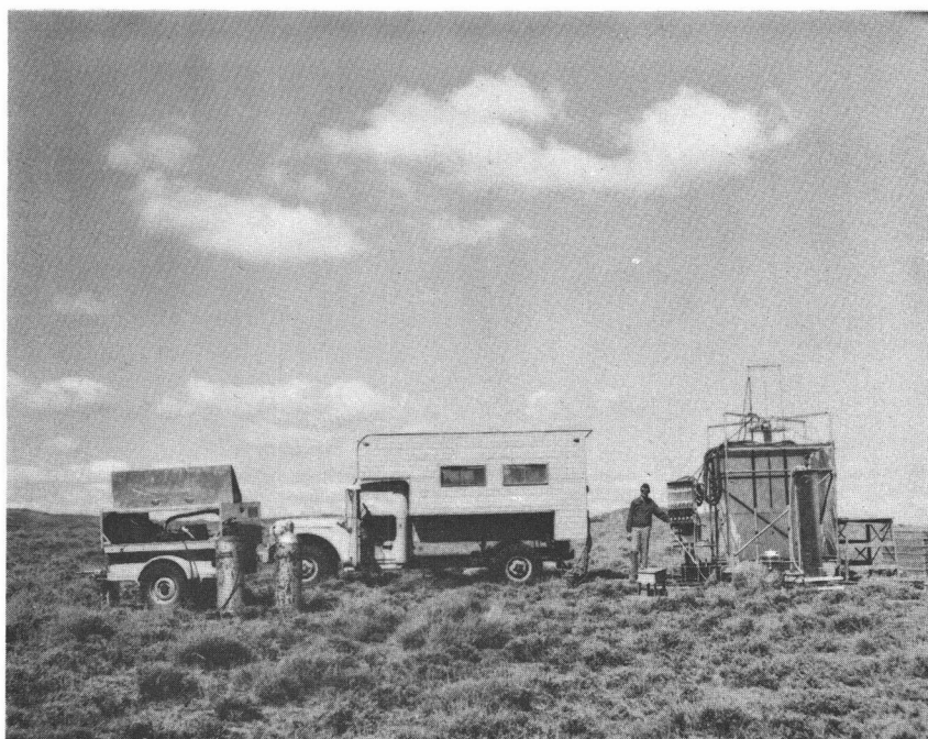
Figure 3. Picture of rainfall simulator, camper for housing instrumentation, and electrical generator which supplied all electrical power.
