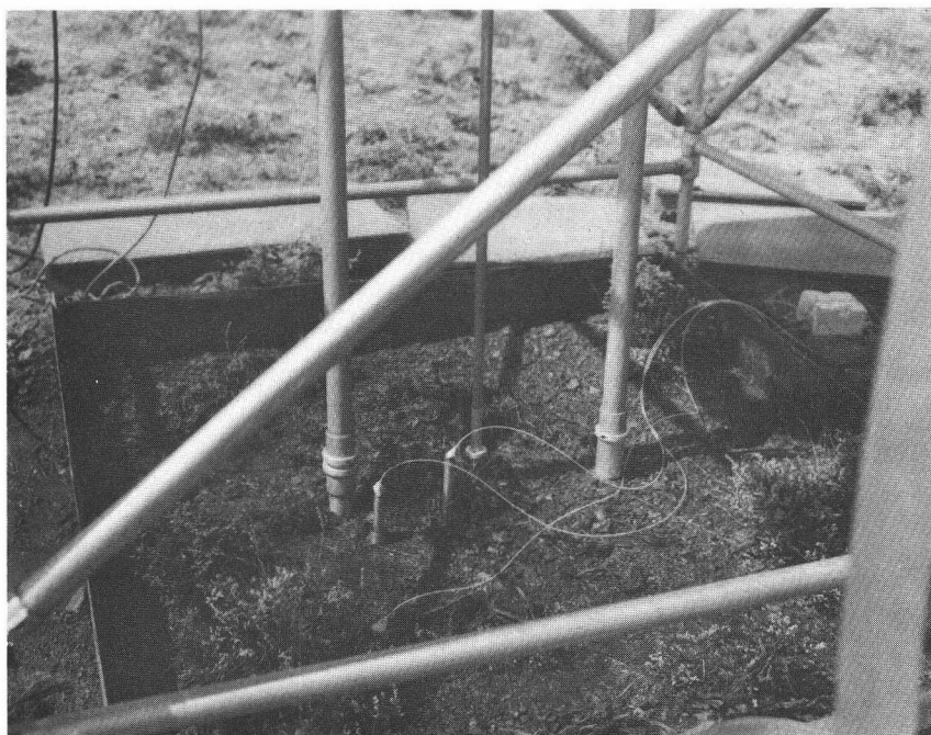
Figure 6. Picture showing an infiltration plot with vertical access tubes for gamma probe and source (see Fig. 4), three tensiometers with nylon tubing going to insulated pressure transducer box, steel border around plot, typical vegetative cover, and pipe frame stand.
