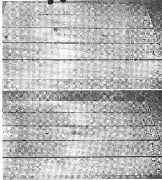
Figure 4. Planks in charge 6 (top), with initial conditions for 9 per cent Emc, checked similarly, but were in kiln 33 hours less than charge 6A (below), with constant conditions for 9 per cent Emc.
