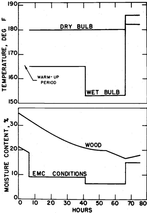
Figure 5. Kiln schedule and rate of drying for fine-grain Douglas fir (Table 1) in charge 9, typical of charges dried to verify results from suggested schedule.
