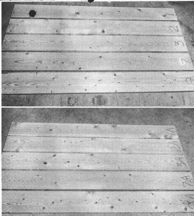
Figure 3. Planks in charge 8 (top), with initial conditions for 9 per cent Emc, had identical drying times and similar checking to charge 8A (below), with initial conditions for 12 per cent Emc.
