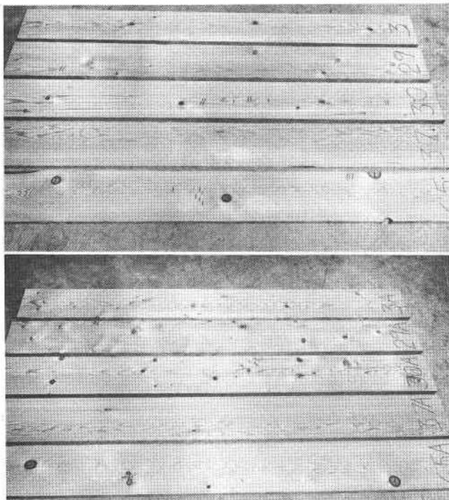
Figure 1. Planks in charge 7 (top), with initial conditions for 9 per cent Emc, checked slightly more, but were in the kiln 26 hours less than charge 7A (below), initially set for 12 per cent Emc.
