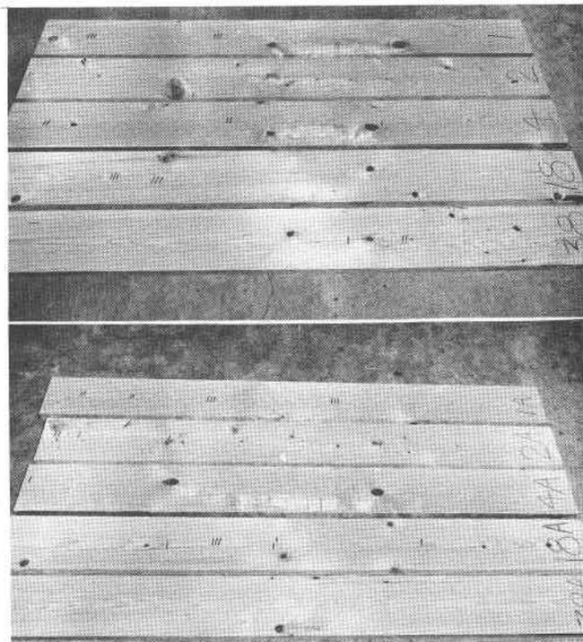
Figure 2. Planks in charge 5 (top), with initial conditions for 12 per cent Emc, checked more and were 15 hours longer in kiln than charge 5A (below), with initial conditions for 9 per cent Emc.
