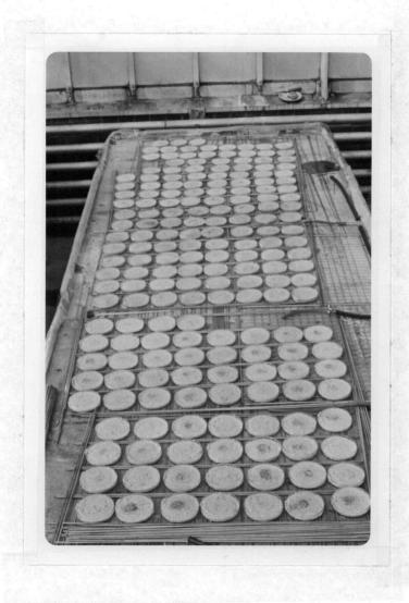
Figure 14. Greenhouse water bath for comparison of herbicides as algicides on the growth of four algae.
