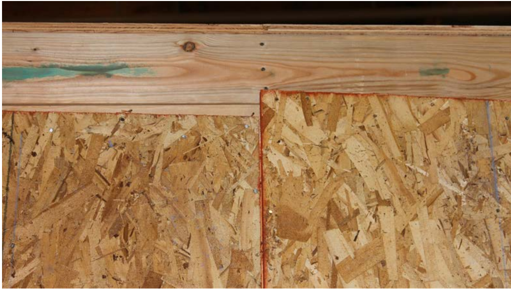
Fig. B.11: Racking of OSB sheathing on shear wall during FAIL2 experiment
