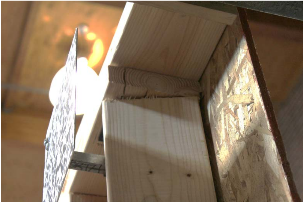
Fig. B.8: SW3 Trial09 top plate splitting at nailed connection
