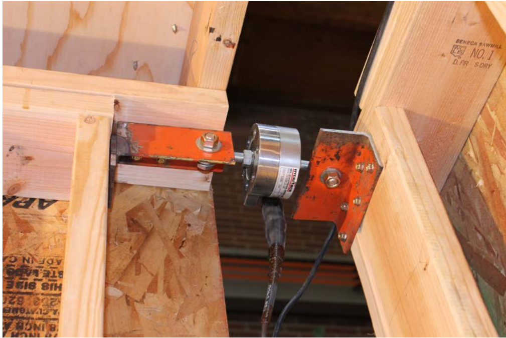
Fig. B.3: Load cell setup for OOP1 experiments
