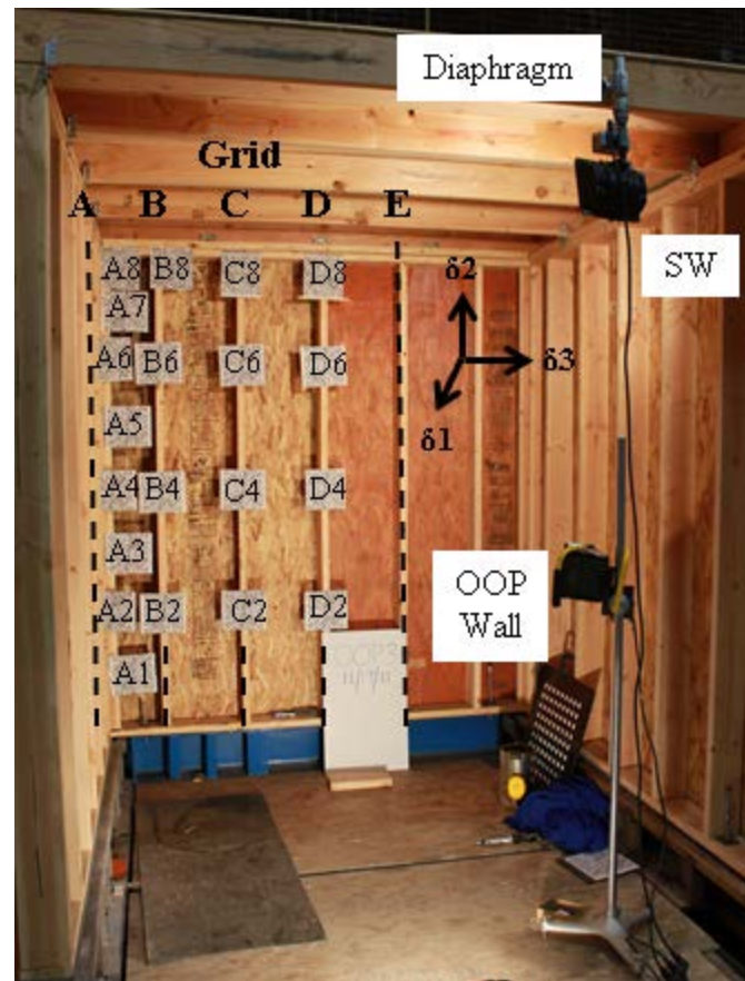
Fig. 2.5: Test setup 2C with grid and targets
