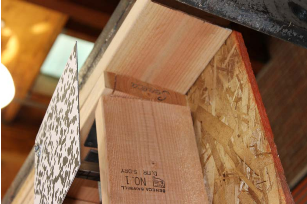
Fig. B.9: SW4 Trial09 top plate splitting at nailed connection
