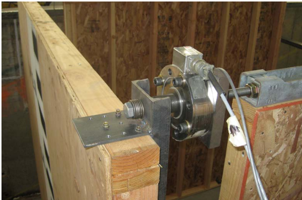
Fig. A.3: Shear wall load cell setup
