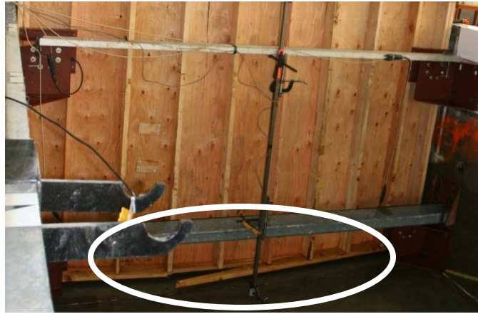
Fig. 1.11: Failed bottom plate of TW 1 (Unanchored, Specimen 1A)
