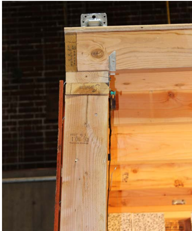
Fig. B.12: Out-of-plane deflection of NE corner during FAIL2 experiment
