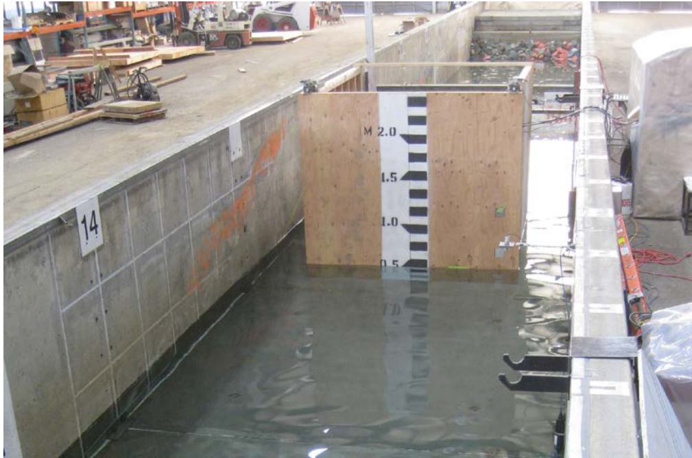
Fig. A.2: ShearWall_1 setup with 8 ft. transverse wall
