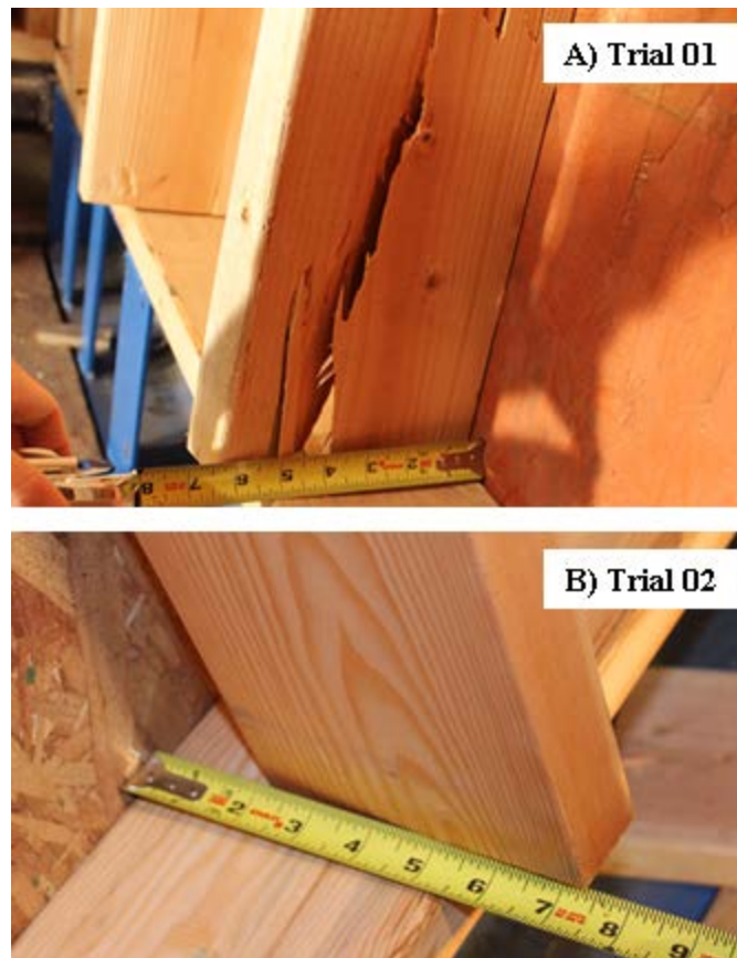
Fig. 2.14: FAIL1 failures: A) Trial 01 stud splitting, B) Trial 02 stud to bottom plate connection failure
