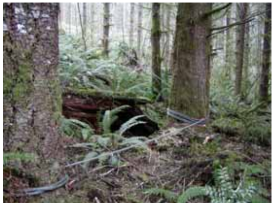
Figure 2. Guyline wraps on a tree and shackled to another tree
