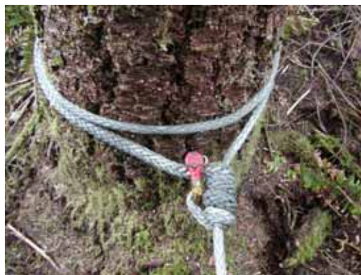
Figure 3. Termination of guyline with shackle
