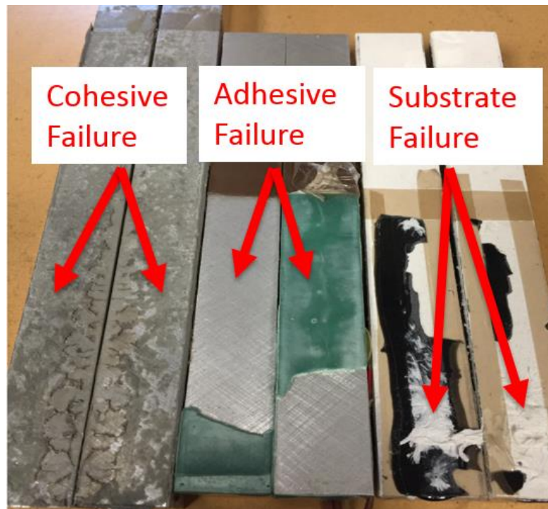
Figure 34 – Adhesive Failure type: Left-Cohesive, Middle-Adhesive, Right-Substrate
