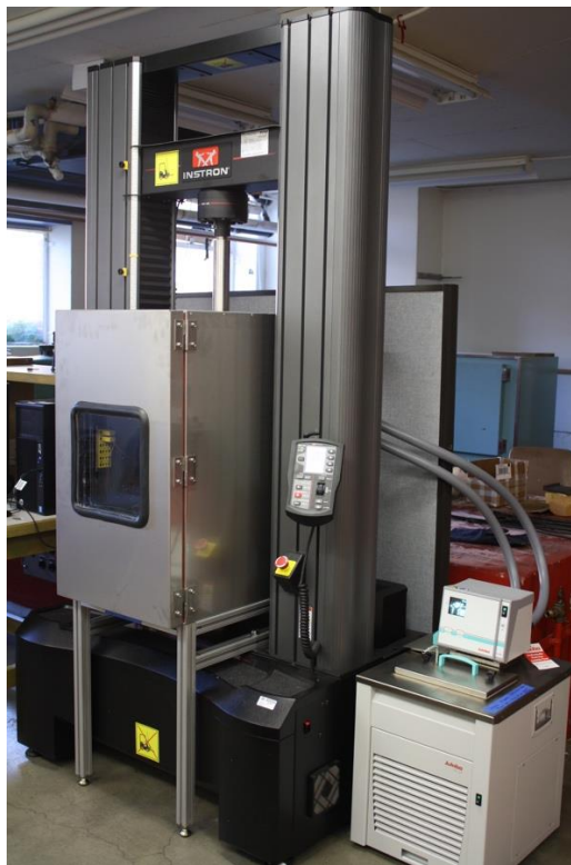
Figure 17 – Temperature chamber built by Meraz at Oregon State University
