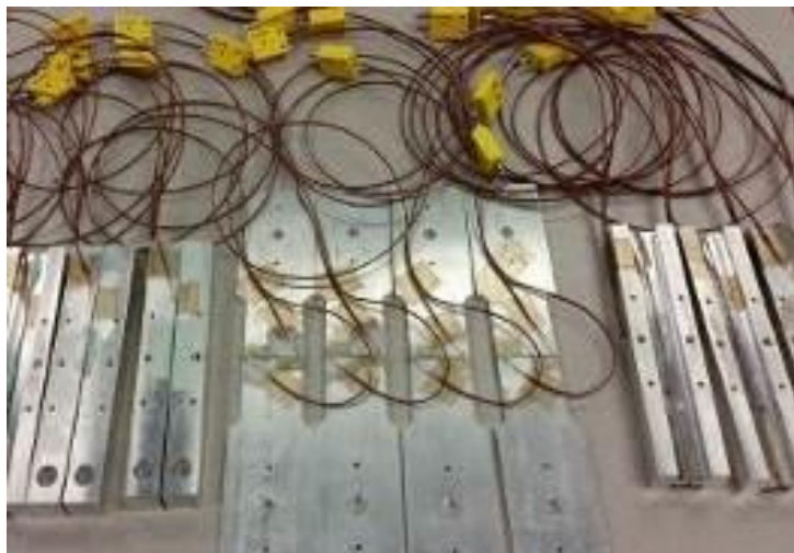
Figure 12 – Thermocouple placement on DCB, DBTS, and SLDCB specimens
