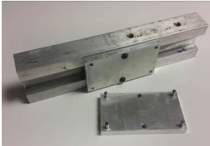
Figure 10 – DCB, SLDCB bond line fixture on an SLDCB specimen
