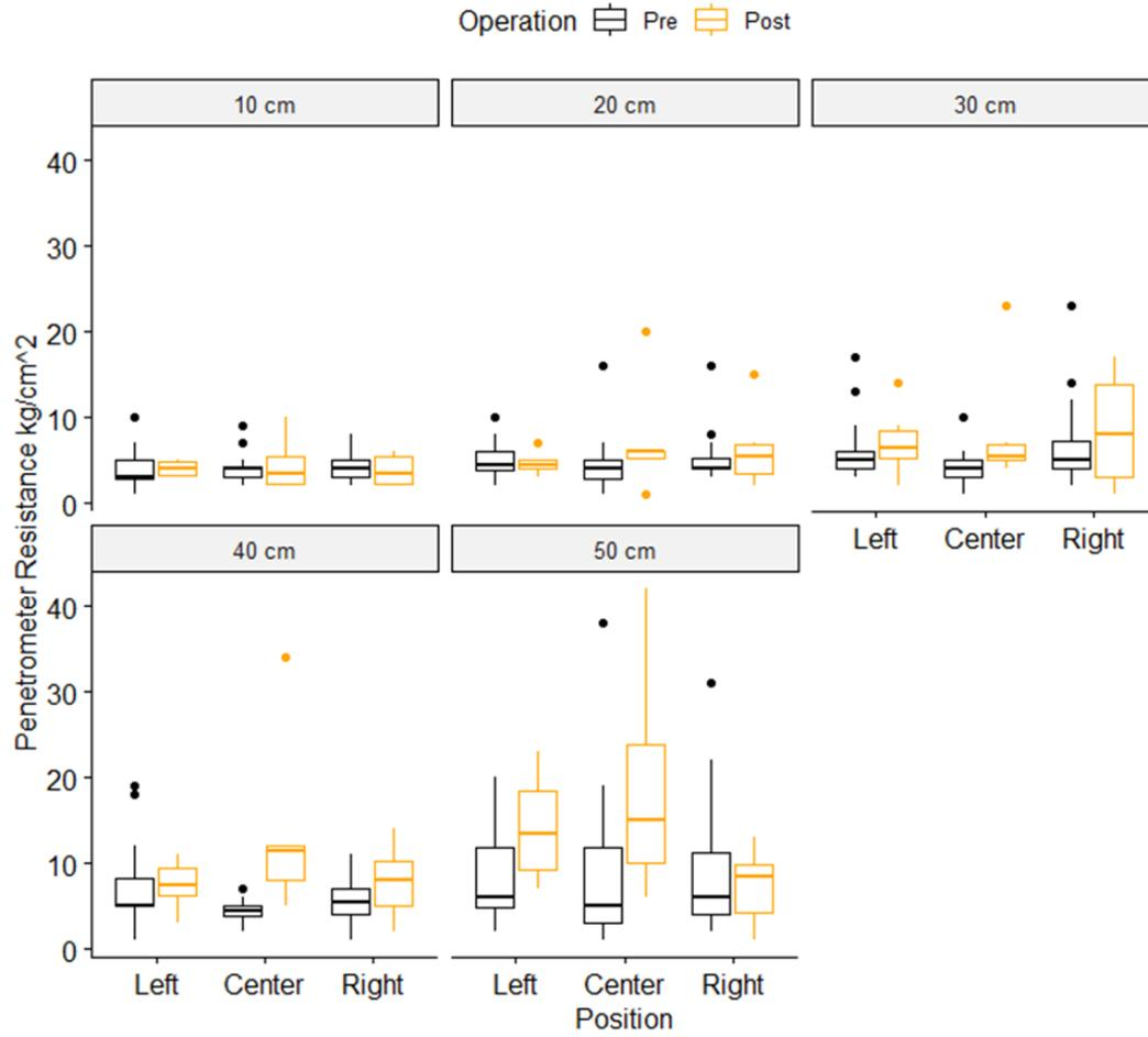
Figure 9: Penetrometer Resistance - Corridor D
