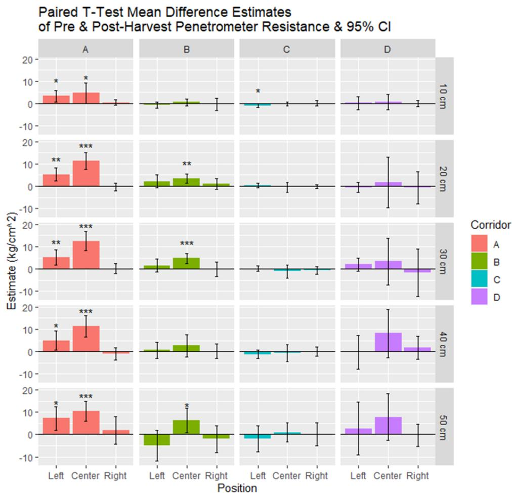
Figure 11: Penetrometer Resistance Paired T-test results
