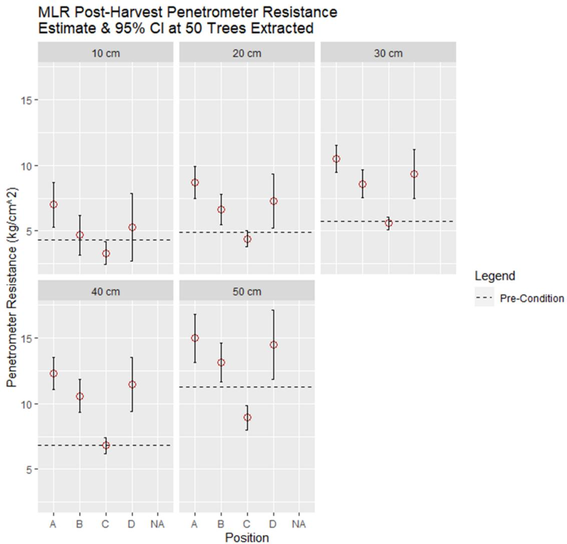
Figure 14: Penetrometer Resistance Prediction - MLR Estimates & 95% CI at 50 Trees Extracted
