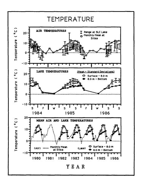
Appendix V. Air temperatures: range at study site (bars) and monthly mean for the highest and lowest daily observations at Sitka, Alaska; lake temperatures: surface (open symbol) and deep water (closed symbol) means recorded over 0.5 m intervals to a maximum depth of 11.7 m (summer 1984-summer 1986); and lake temperature overlayed on Sitka monthly mean air temperatures (broken line) for the entire study period (1980-1986).
