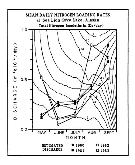
Appendix XI. Mean daily total nitrogen loading (isopleths) with respect to mean monthly lake discharge and time of year. Monthly mean discharges estimated for summer months prior to 1984 were plotted on the isopleth model to calculate monthly total nitrogen loading rates for Sealion Cove Lake, Alaska.
