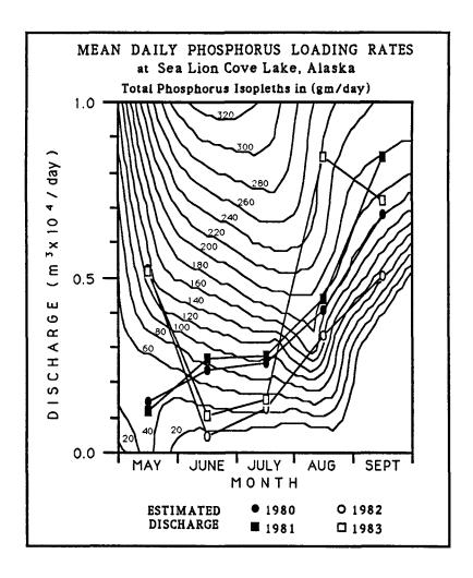
Appendix X. Mean daily total phosphorus loading (isopleths) with respect to mean monthly lake discharge and time of year. Monthly mean discharges estimated for summer months prior to 1984 were plotted on the isopleth model to calculate monthly total phosphorus loading rates for Sealion Cove Lake, Alaska.
