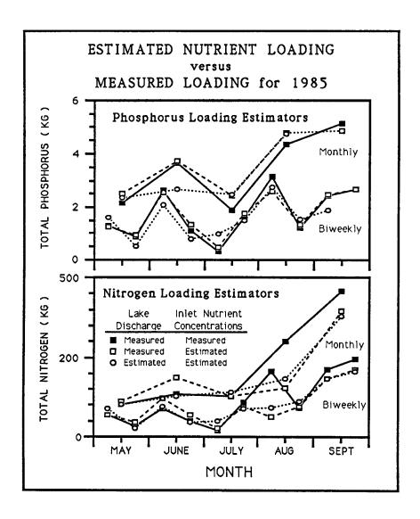
Appendix XII. Test runs for the nutrient loading (isopleth-regression) model comparing results obtained with estimated parameters (open symbols) to an independent estimate calculated directly from measured parameters (closed symbols).
