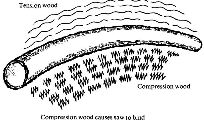
Figure 17.—Compression and tension wood
