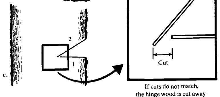
Figure 5.—(a, b, and c) Types of undercuts; (d) the first cut using an axe to check direction-of-fall; and (e) matching the cuts.
