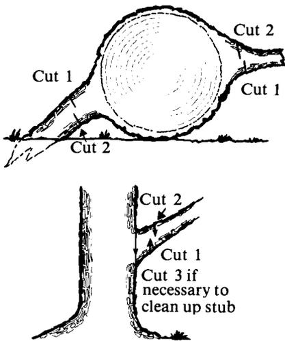
Figure 22.—Cut limbs by cutting compression wood first as shown (top) on a log with limbs, and (bottom) on a standing tree.
