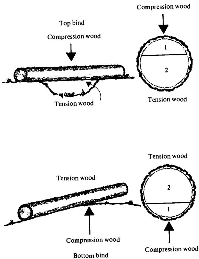
Figure 18.—Determining top bind and bottom bind for bucking small logs.
