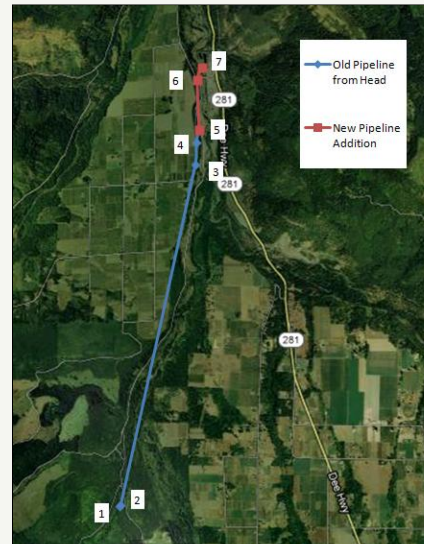
Map of the new pipeline route where point 1 corresponds to the Tony Creek screen house (and penstock head), point 5 the splice into the old pipeline, point 6 the west side of the new bridge, and point 7 the turbine house. GPS measurements are overlaid on a satellite image.
