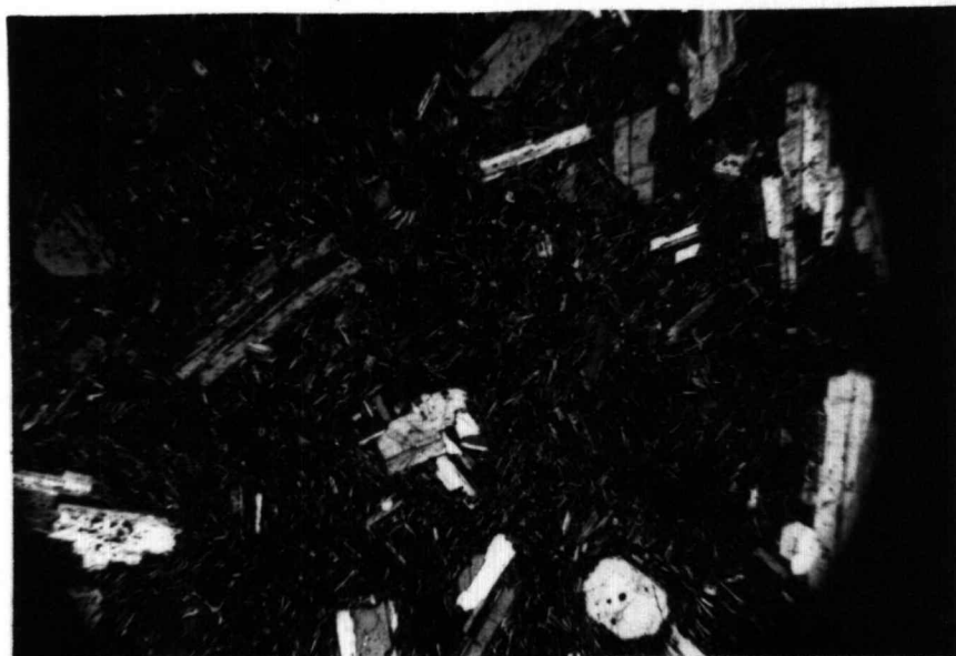
Figure 21. Photomicrograph, basalt porphyry with plagioclase and augite phenocrysts, Goble Volcanics. Note glass (circular areas, lower center and upper left, black.) Crossed polars. (Locality 277, Rocky Point.)
