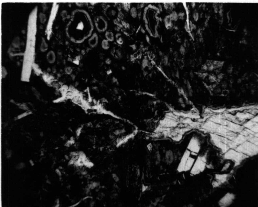
Figure 60. Photomicrograph, pebbly calcareous volcanic sandstone, lower member, Keasey Formation, Nehalem River. Note vesicular basaltic rock fragments with devitrified palagonite lining vesicles. Sparry calcite cement. (locality 143B.)
