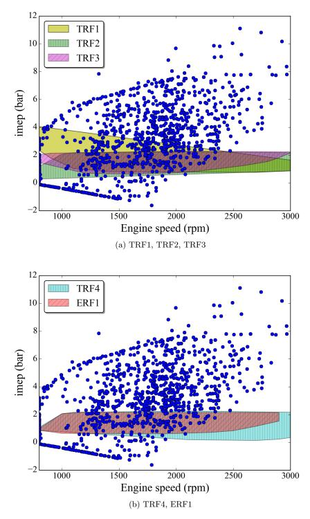
Figure 6: Operating envelopes for ternary TRF and ERF mixtures at CR = 9.5 and naturally aspirated inlet conditions over FTP-75 driving cycle.
