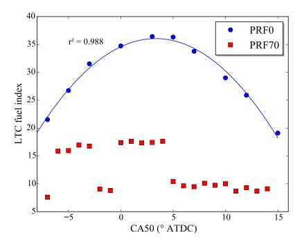
Figure 10: LTC fuel index for PRF0 and PRF70 with varying target CA50 value. Symbols indicate the actual points and the line is a quadratic fit with the coefficient of determination given as  $r^2$ . PRF70 results have no obvious correlation.
