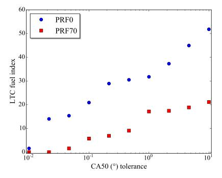
Figure 11: LTC fuel index for PRF0 and PRF70 with varying CA50 tolerance, centered around  $3^{\circ}$  ATDC. Note the logarithmic scale of the the horizontal axis.
