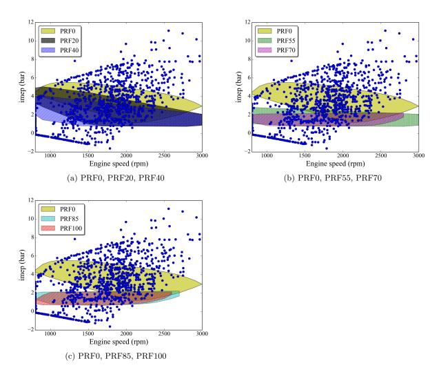
Figure 4: Operating envelopes for PRF mixtures at CR = 9.5 and naturally aspirated inlet conditions over FTP-75 driving cycle. PRF0 (*n*-heptane) is repeated in each figure for perspective.
