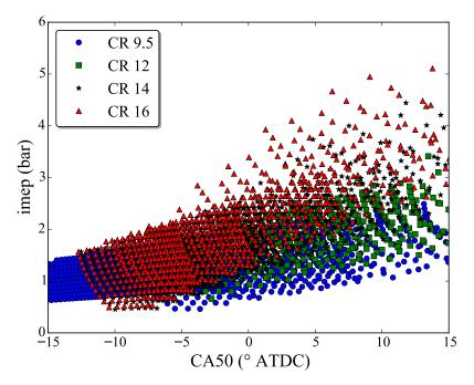
Figure 9: PRF70 operating range given in impe as a function of CA50 value, with varying compression ratios (as shown), engine speeds over 800–3000 rpm, equivalence ratios of 0.1–0.45, and initial temperatures over 310–600 K.
