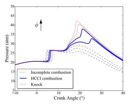
Figure 2: Representative pressure traces for PRF0 (*n*-heptane) HCCI combustion at CR = 9.5, initial temperature of 330 K, initial pressure of 1 atm, 1400 rpm, and varying equivalence ratios, demonstrating knocking combustion, normal combustion, and misfire.
