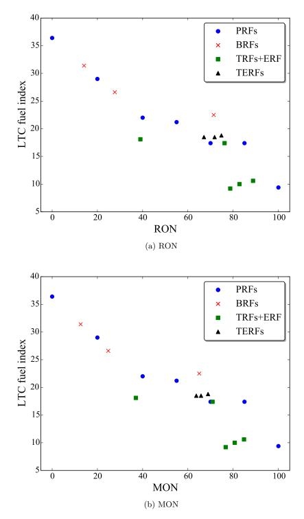
Figure 8: Correlations between LTC fuel index and RON/MON, with symbols indicating the different fuel mixtures.
