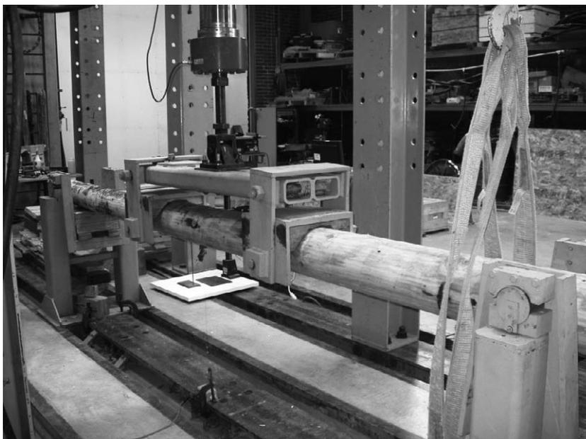
Figure 1.—Photograph showing a pole in the test setup.
