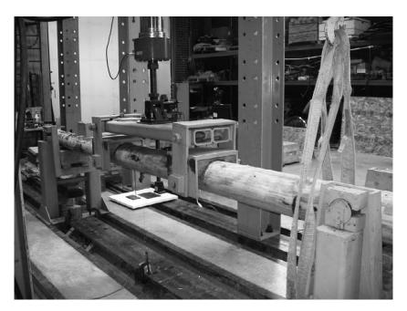
Figure 1.—Photograph showing a pole in the test setup.
