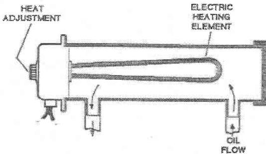
Figure 4. Electric Heat Exchanger
