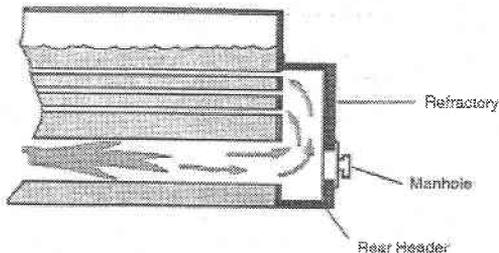
Figure 2. Dry Back SM Boiler
