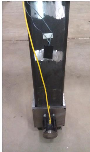
Figure 3.7: Strain gage adhered to load cell side of column assembly
