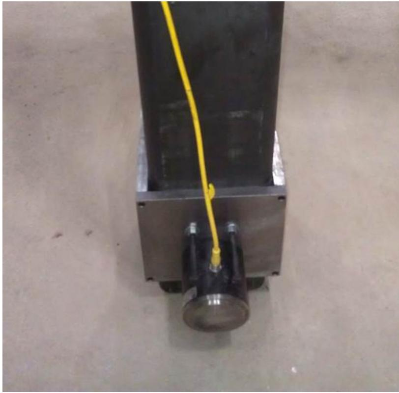
Figure 3.11: Photograph of stainless steel sleeve used to attach the load cell to the column assembly. Manufactured to allow sleeve to move up and down the column.
