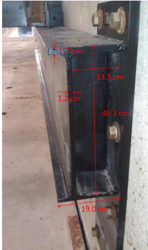
Figure 3.10: Photograph of one of the supports of the column assembly on the wave flume wall. Identical support is located on the opposite wall. Dimensions are included.
