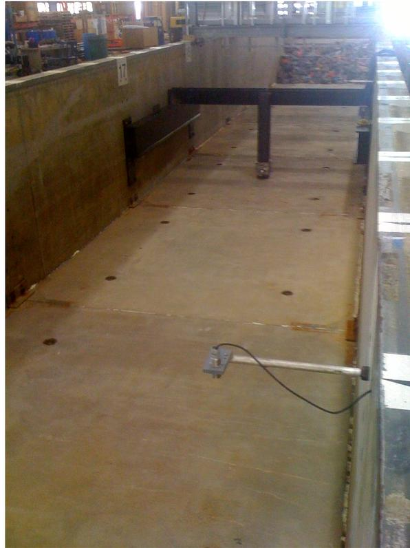
Figure 3.2: Ultrasonic wave gage installed in wave flume. Location uswg3 is shown.
