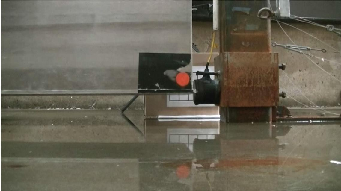
Figure 3.26: Video frame of In-Air Longitudinal Test using Panasonic HD camera. The view point of this frame was used to track the velocity of the debris as it swung and collided with the load cell. The orange circle painted in the bottom right hand corner of the specimen was used to track debris movement.
