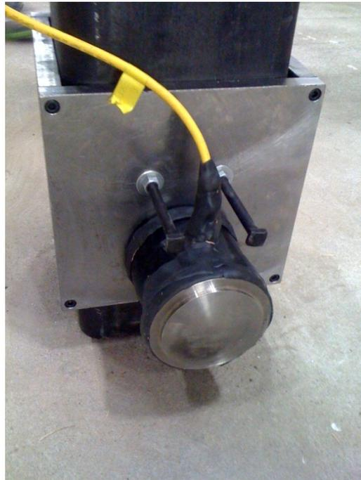
Figure 3.5: Waterproofing material applied to CLC-300K load cell
