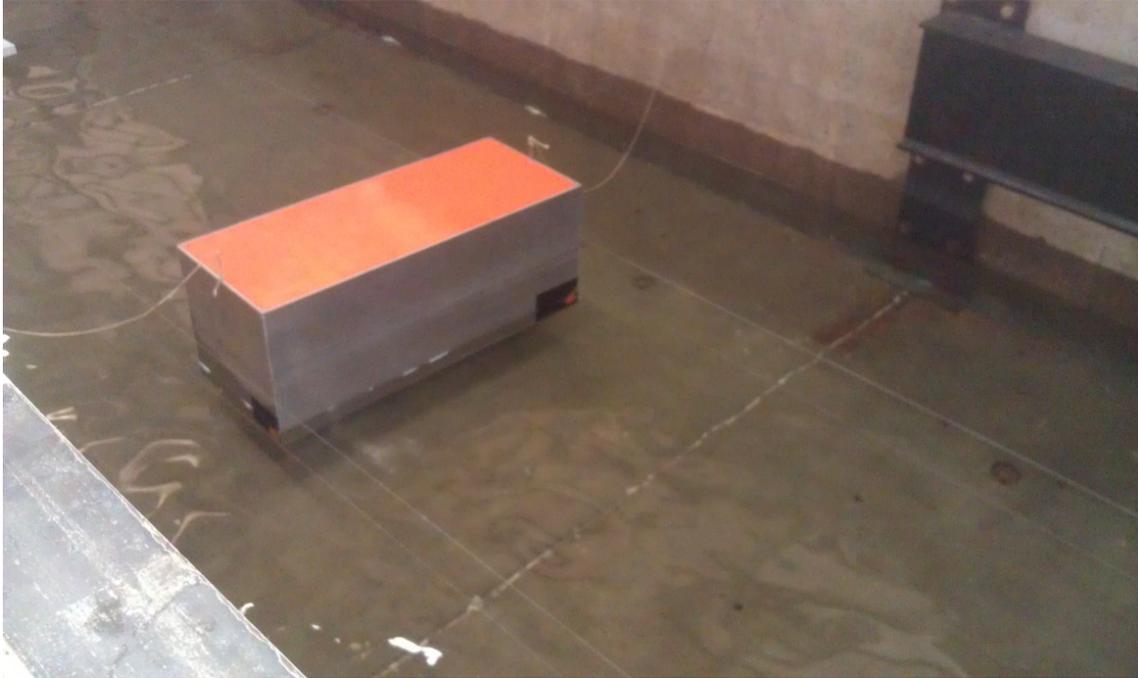
Figure 3.19: Photograph of guide wire setup for transverse in-water test. The tethers shown in the photograph were used to position the specimen for each trial as well as maintain orientation during each trial.
