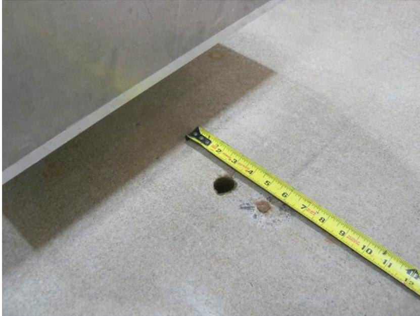
Figure 3.42: Measuring tape used to measure pullback distance,  $X$ .
