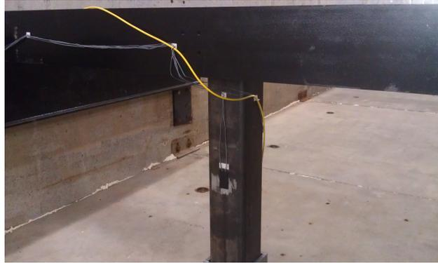
Figure 3.6: Strain gage adhered to side opposite of load cell on column assembly
