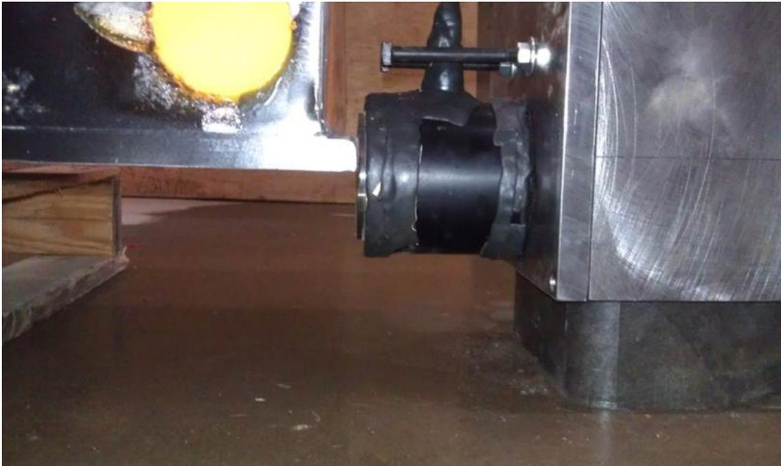
Figure 3.41: Resting point for debris specimen relative to load cell during In-Air longitudinal aluminum test.
