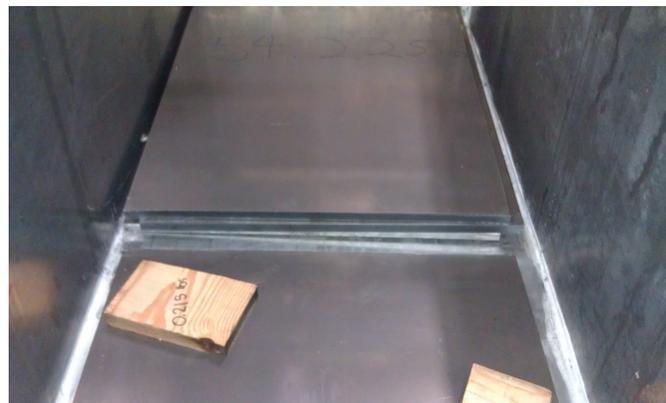
Figure 3.17: Another view of nonstructural mass inside aluminum specimen. Photograph is shown after in-air trial is performed. Steel plates are shown to have shifted to the front of the specimen.
