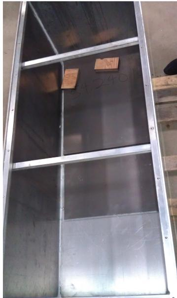
Figure 3.16: Photograph of nonstructural mass placed in aluminum debris specimen. Four hot rolled steel plates with wooden block supports are shown.
