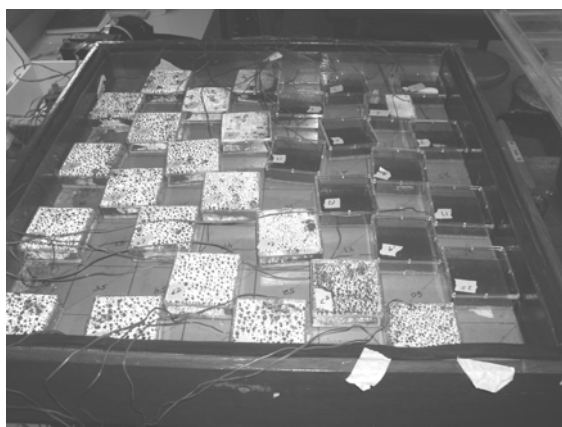
Figure A1.1 – Example of a two-way thermogradient plate with germination boxes and temperature monitoring thermocouples. Approximate size of plate is 1\text{m}^2 .
