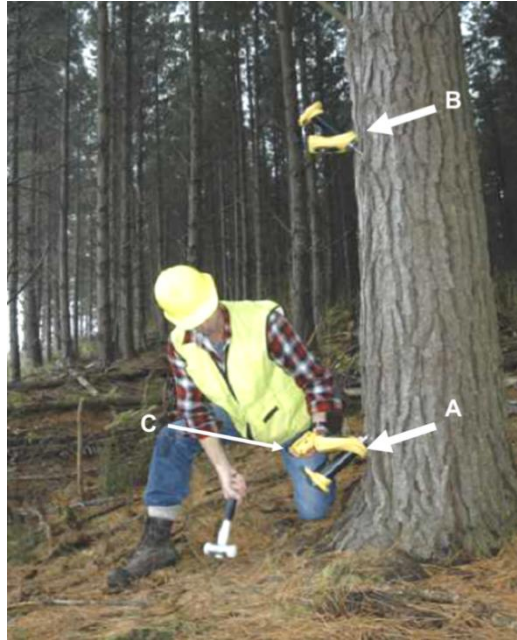
Figure 1. Measurement of acoustic velocity with the Hitman ST300. (A) Transmitter probe (B) Receiver probe (C) Personal digital assistant (Fibre-gen.com, 2015).
