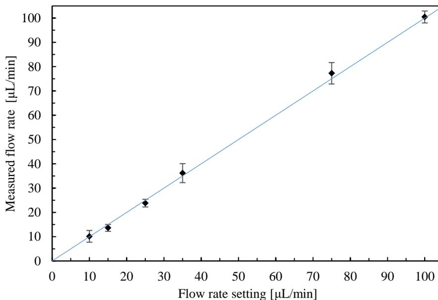
**Figure 18:** Calibration curve for syringe pump flow rate. Data points shown are an average of five trials at each flow rate. Error bars represent a 95% confidence interval. The blue line represents exact unity between measured flow and syringe pump flow rate setting.
