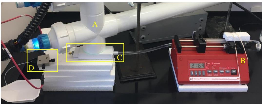
**Figure 8:** Experimental apparatus for continuous flow trials. Equipment includes 254 nm light source (A), syringe pump (B), 3D printed reactor (C), and UV-vis flow cell (D).
