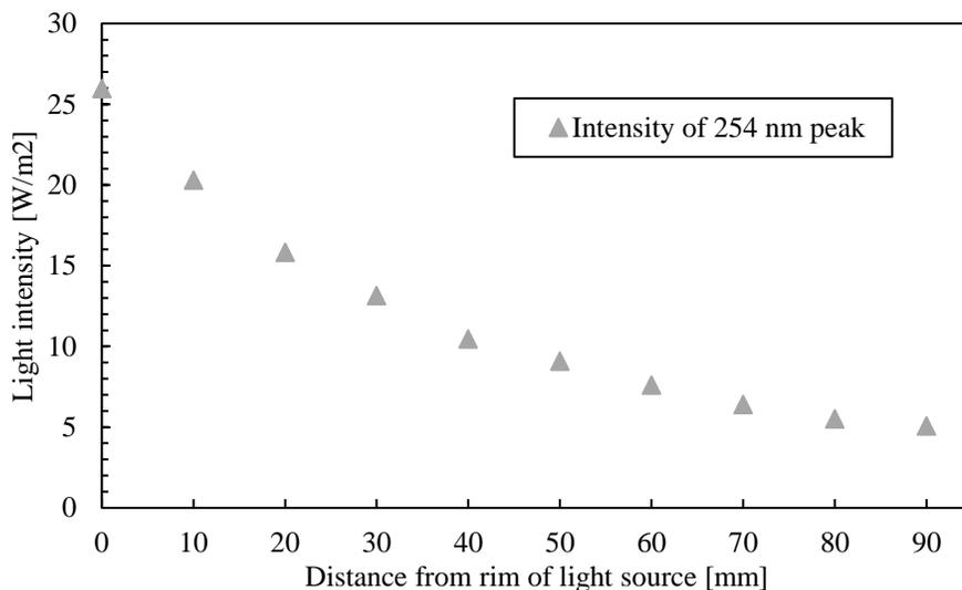
**Figure 17:** Relationship between UV light intensity and distance from light source. Light detector was covered with a single crystal sapphire slide to simulate experimental conditions in the continuous flow reactor. Intensity shown is an integration from 251 – 255 nm.
