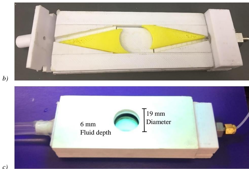
**Figure 7:** 3D printed continuous flow reactor. a) SOLIDWORKS exploded model of 3D printed components, including part labels. b) Partially constructed reactor showing fluid flow channel. c) Fully constructed and functioning reactor during an acetaminophen photolysis trial.
