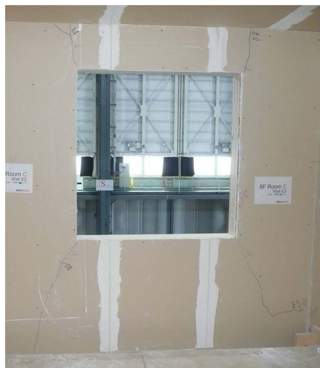
Fig. 20. Story 6, Wall E2; cracks develop all the way through panel for all corners after Seismic Test 5
