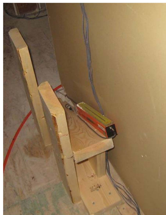
Fig. 3. Diagonal deformation measurements using stringpot
