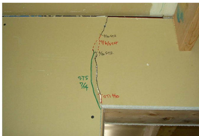
Fig. 16. New crack on Wall 2A, Story 7 (over door opening) after Seismic Test 5
