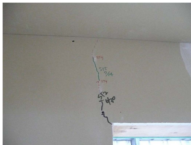
Fig. 19. Story 6, Wall E1; cracks develop all the way through panel after Seismic Test 5
