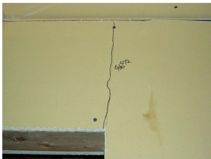
Fig. 10. No new crack on Wall 2A, Story 7 (over door opening) after Seismic Test 3; the crack shown was developed during Seismic Test 2
