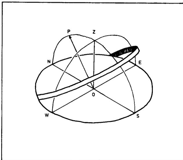
Figure 1. Aerial projected view of a shade ring. The pyranometer is at O. The shade ring is in the plane perpendicular to the polar axis OP and is moved up and down the axis with the seasons. The ring position shown is for 53°N when the solar declination is 16° (6 May or 8 August).
