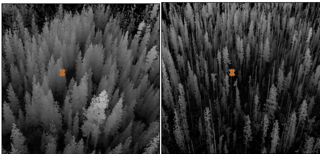
Figure 3.2. Terrestrial laser scanner data of unburned and burned forest measured June 2012 (shown as a bird's-eye perspective of both forests sites with the station location located under the orange X in each image).
