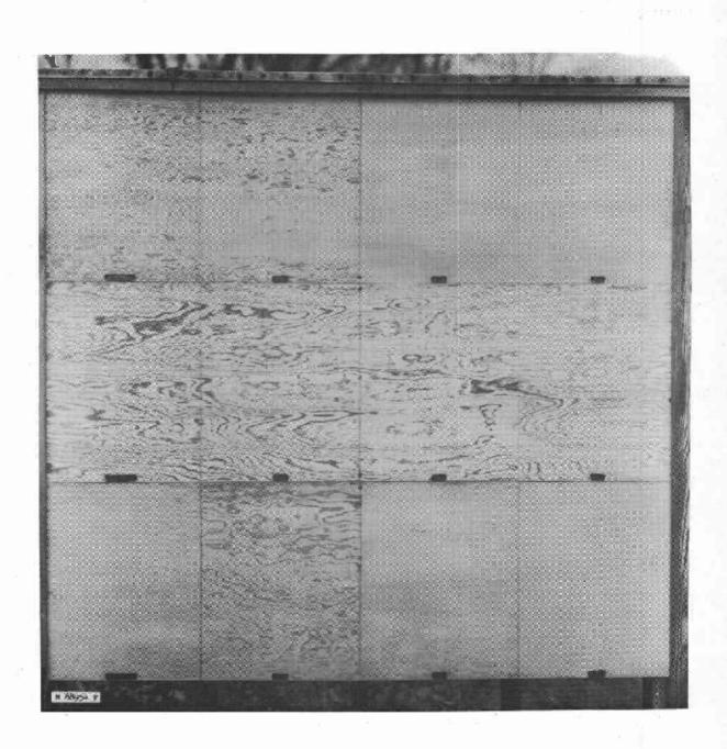
Figure 7.--Condition of paint on plywood covered with resin-impregnated paper in the 1944 tests after exposure vertically facing south for 71 months at Madison, Wis. The primers and paints and their arrangement on the test areas were the same as they were on the plain plywood shown in figure 6.
