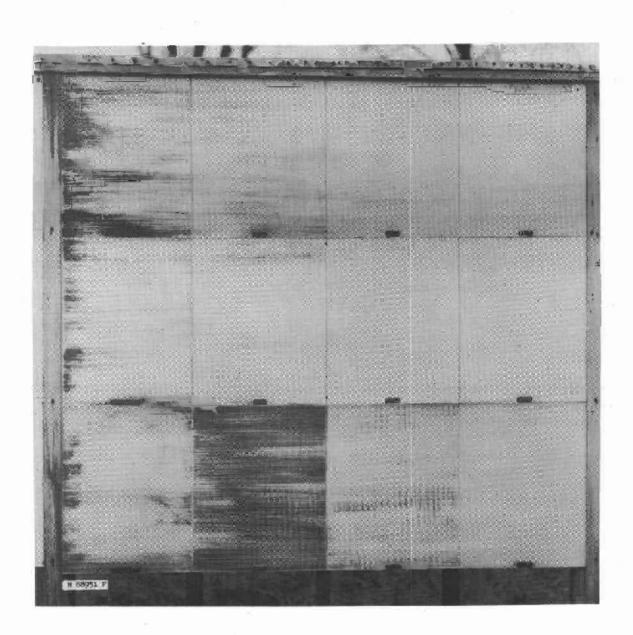
Figure 8.--Superior performance of paint on striated Douglasfir plywood as compared with plain plywood. Both views were taken on parts of the same building in southern Arizona that were last painted about 2 years previously with the same kind of paint. Note that the striated plywood shows no face checking as well as superior coating integrity, whereas the plain plywood checked very badly.
