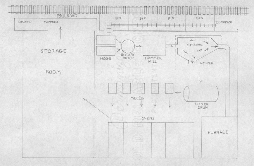
SCALE I"=10' FLOOR PLAN OF CORK MILL.
