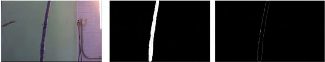
Figure 4.1: Left to right shows the actual RGB image, segmentation mask, and the edges of the branch.
