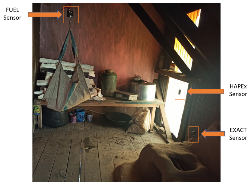
Figure 1.1: Sensor suite deployed in the a Nepalese household.
