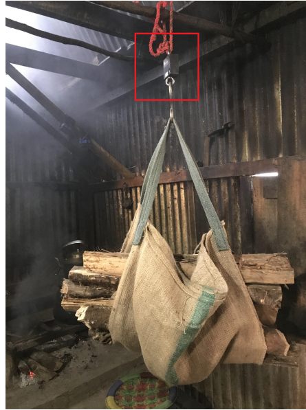
Figure 2.5: A FUEL system installed in one of the Nepalese Households. Red square indicates the actual FUEL sensor.
