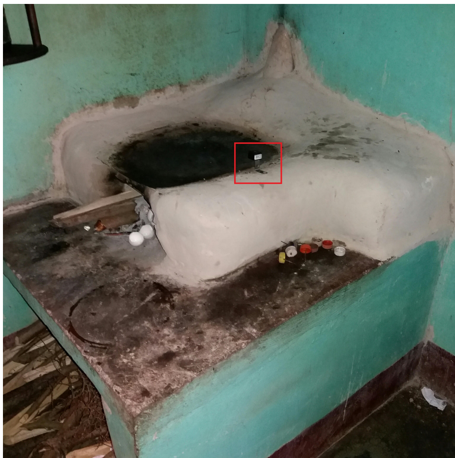
Figure 10: EXACT sensor attached directly to a stove using U-nails.
