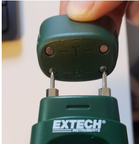
Figure 25: Moisture Meter Battery Test
