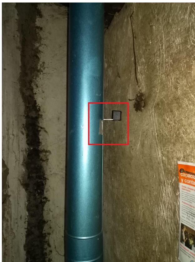
Figure 6: Metallic tape used to attach the EXACT sensor to a chimney. The tape should be rated to at least 100C.
