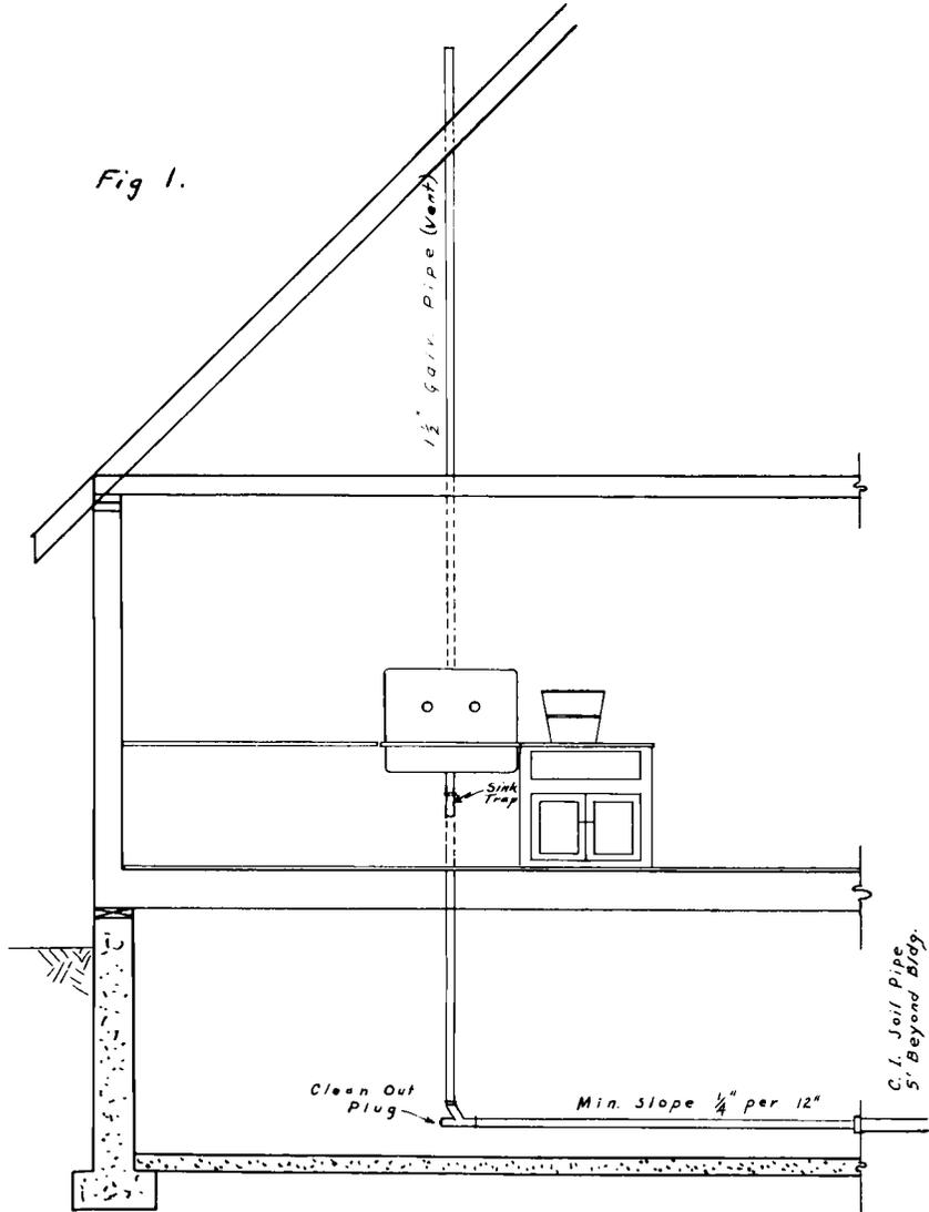
A Simple Sink and Drain Installation
