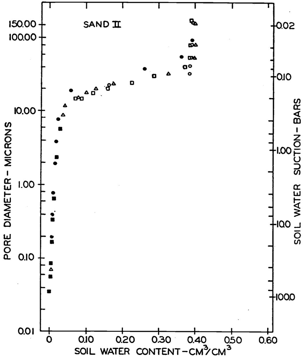
Figure 3. Soil water characteristic curves determined by mercury intrusion ( $\Delta$ ,  $\square$ , and  $\blacksquare$ ) and by the pressure plate apparatus ( $\bullet$ ). The data obtained by mercury intrusion represent three samples showing the reproducibility of this technique. These data were collected during part of one day. About one week of work, distributed over a one month period, was required to obtain the 9 pressure plate points. Results from the two procedures agreed quite well.
