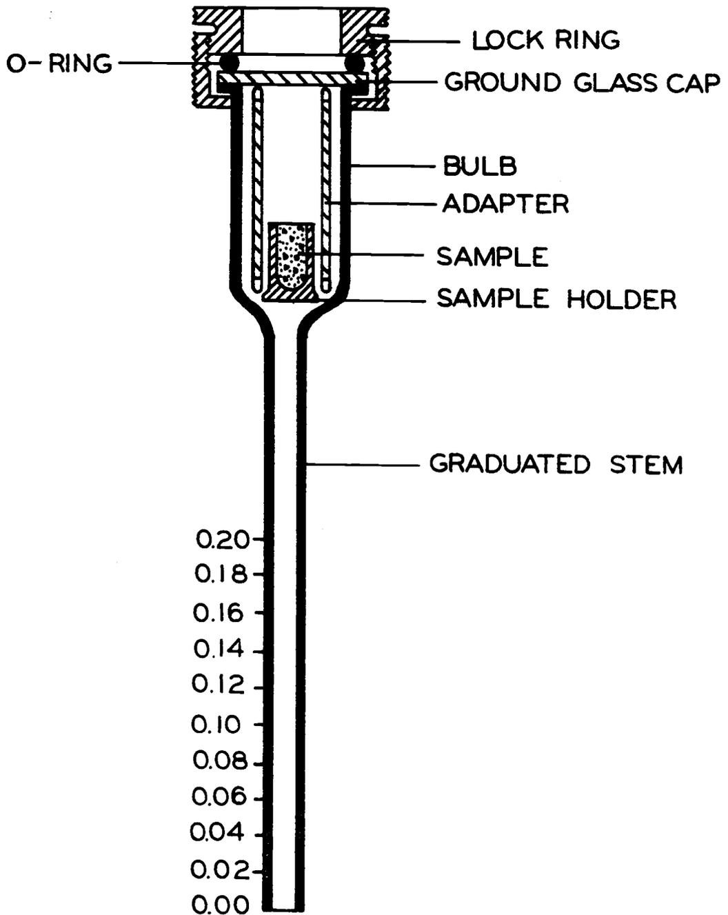
Figure 1. Penetrometer for the mercury intrusion porosimeter. The sample holder consisting of a glass cup with holder was developed for the experiments described. A contained sample was required for control of the packing of the material used.
