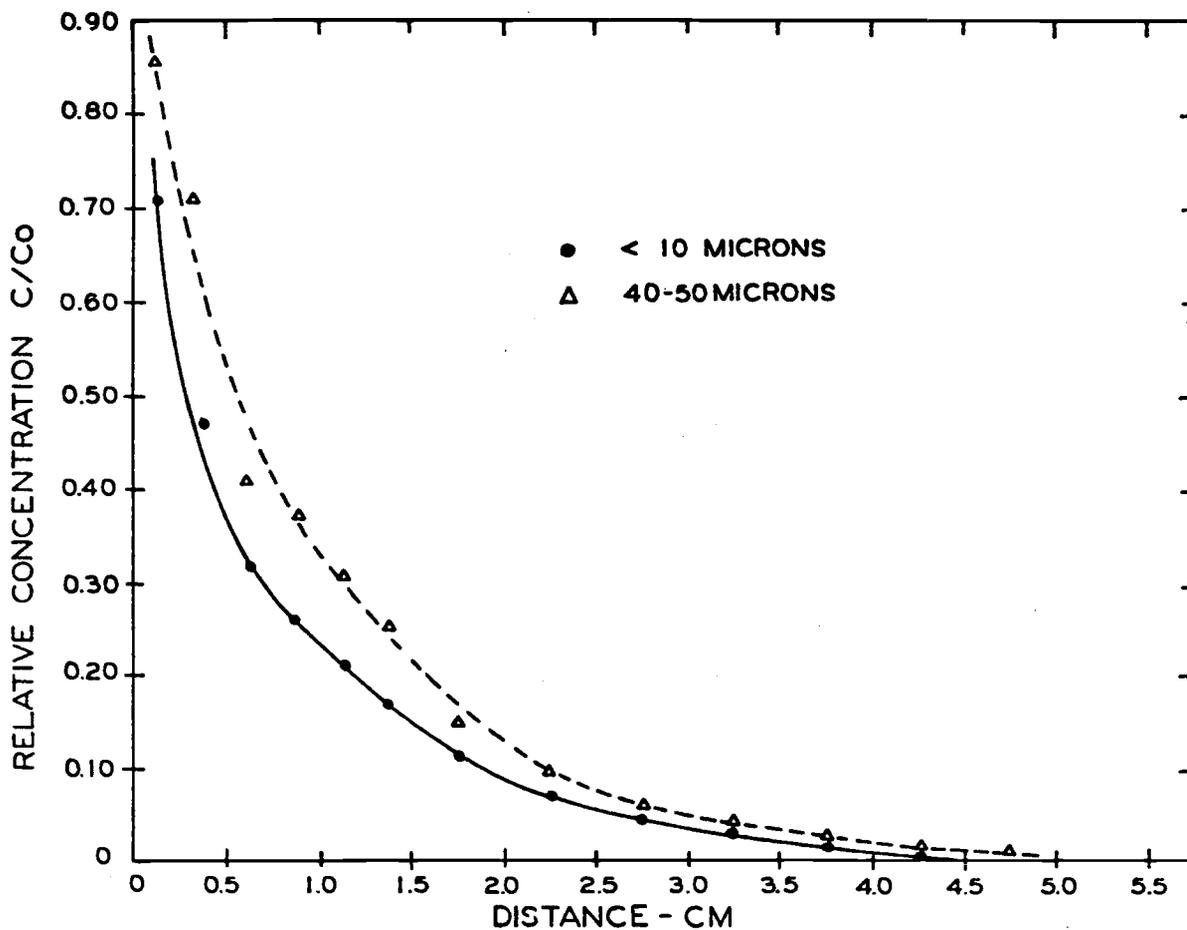
Figure 7. Distribution of 2-4,D in columns made up of glass beads. The concentration at the face of the columns was maintained constant. The graphs show the influence of pore size on diffusion. The rate of advance decreased as pore size decreased. Total pore space was the same in all samples. Diffusion coefficients calculated from these curves allow an evaluation of the equation stated in the text.
