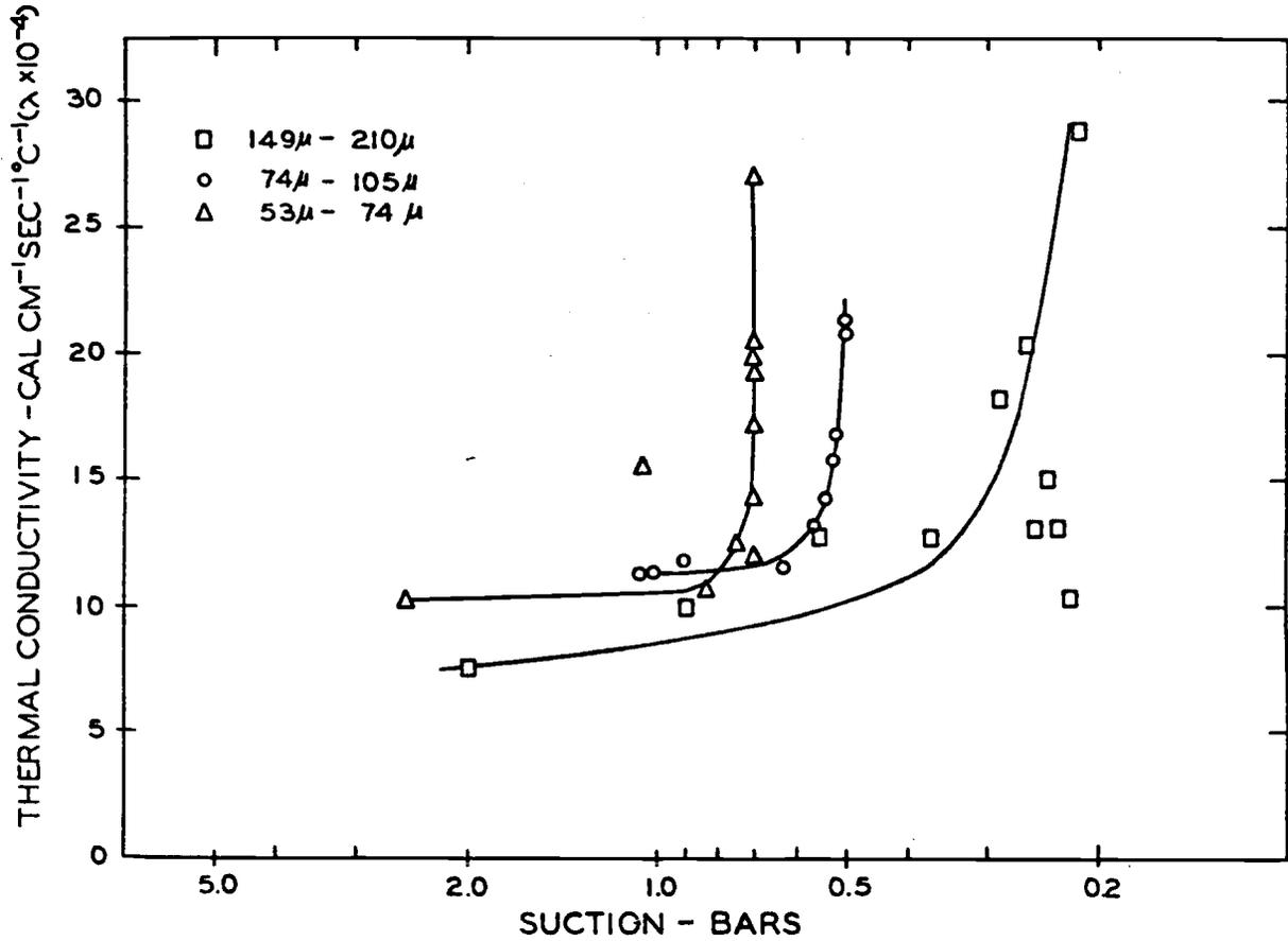
Figure 6. Thermal conductivity of three size classes of glass beads as a function of water suction. The rapid decrease of the thermal conductivity of the largest size class at about 0.2 bars indicates that most of the water drains at this suction. To remove water from the smaller size classes progressively higher suctions are required.
