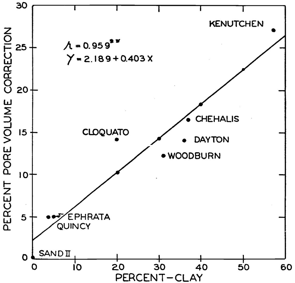
Figure 5. Degree of transposition required to make the mercury intrusion data coincide with the pressure plate data in percent pore volume as a function of the clay content of the soil.
