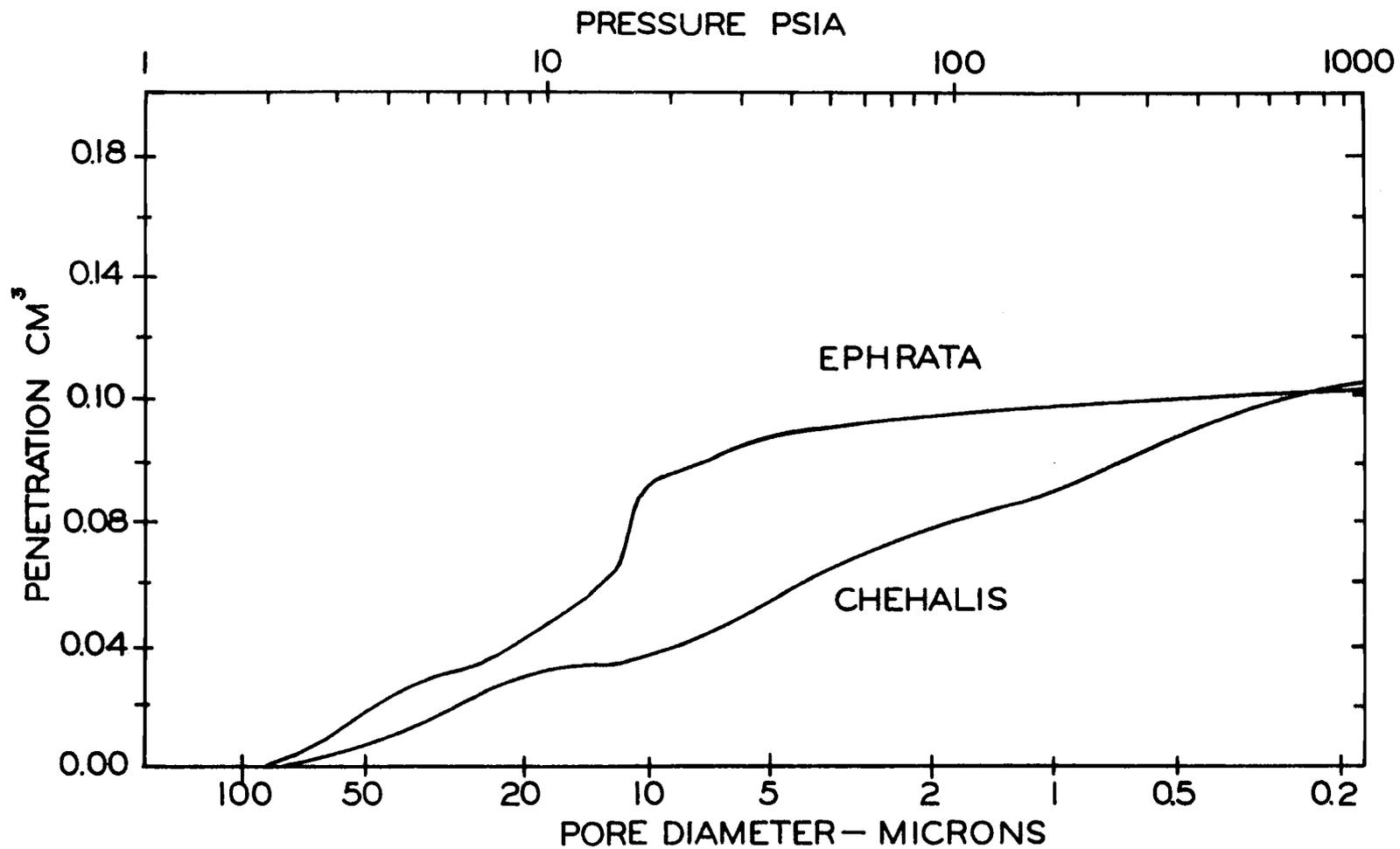
Figure 2. Pore size distribution obtained by mercury intrusion for Ephrata loamy sand and Chehalis loam. The graphs shown represent pore size accumulation curves. The actual pore space in a given pore size increment can be obtained from the ordinate which shows penetration in cm<sup>3</sup> of mercury.
