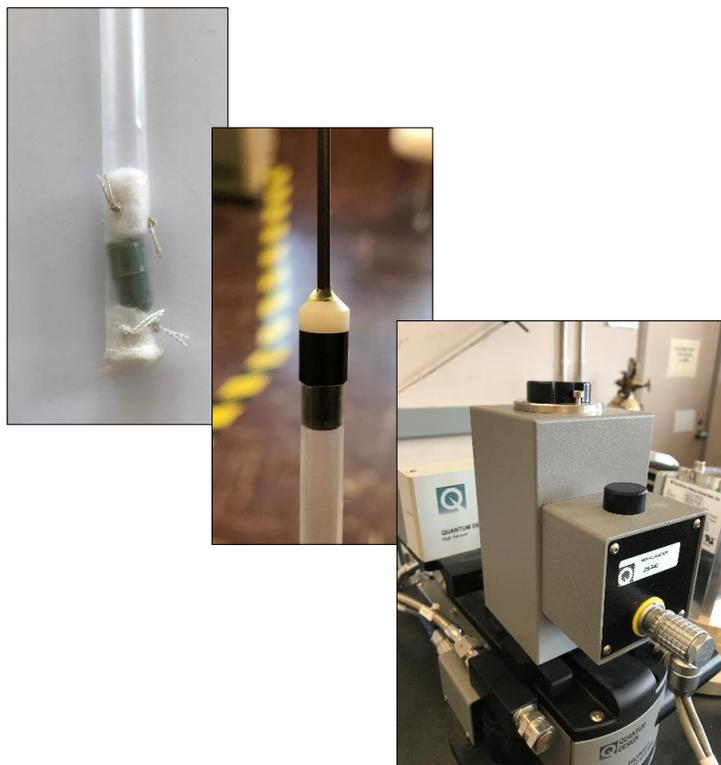
Figure 2.7: Sample preparation for ACMS: sample powders are packed into a straw (left), fitted to a sample rod (middle), and inserted through the DC servo motor (right).
