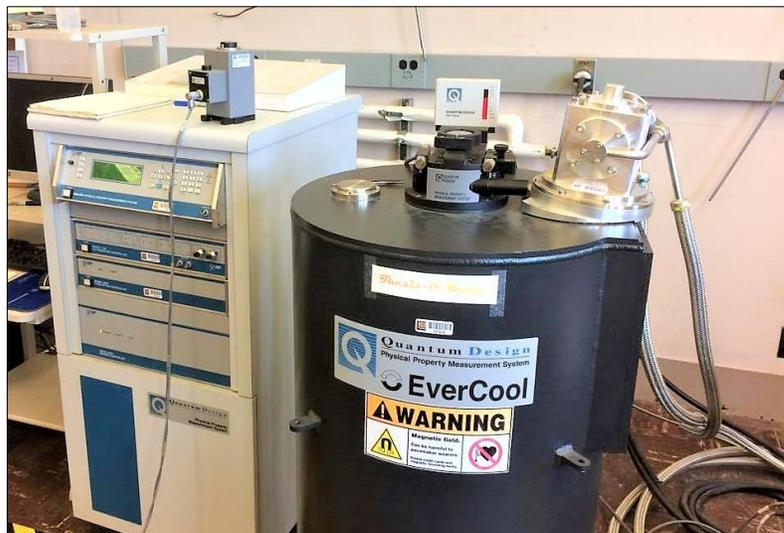
Figure 2.6: The Quantum Design Physical Property Measurement System (PPMS). The Model 6000 controller is housed in the white cabinet (left), while the sample chamber is housed in the He containment dewar (black, center). The cryopump (He level control via a second stage and condenser) is integrated into the dewar, and is connected to a compressor (not shown). Not shown: Scroll pump housing unit (temperature control), diaphragm pump housing unit (pressure control).
