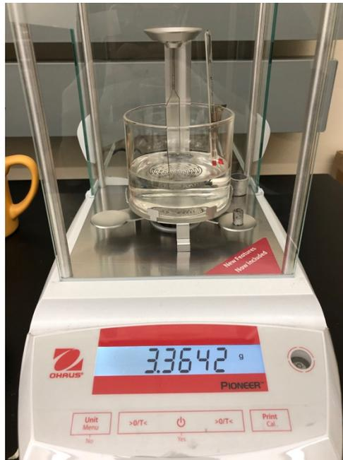
Figure 40: Ohaus Pioneer Archimedes density measurement kit
