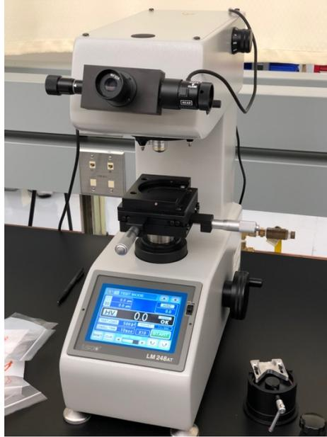
Figure 47: LECO LM 248AT microhardness tester
