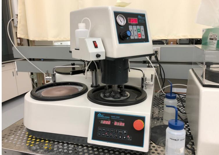
Figure 44: NANO-2000T Grinder-Polisher by Pace Technologies used for grinding/polishing mounted samples.
