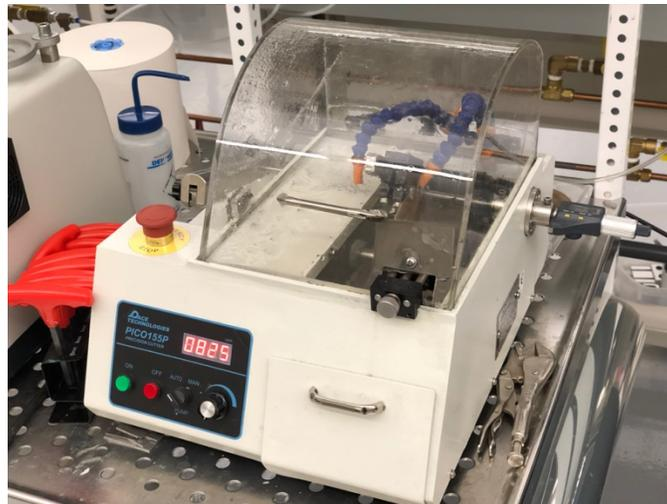
Figure 41: Pace Technologies PICO155P precision cutting saw for cross sectioning the specimens.
