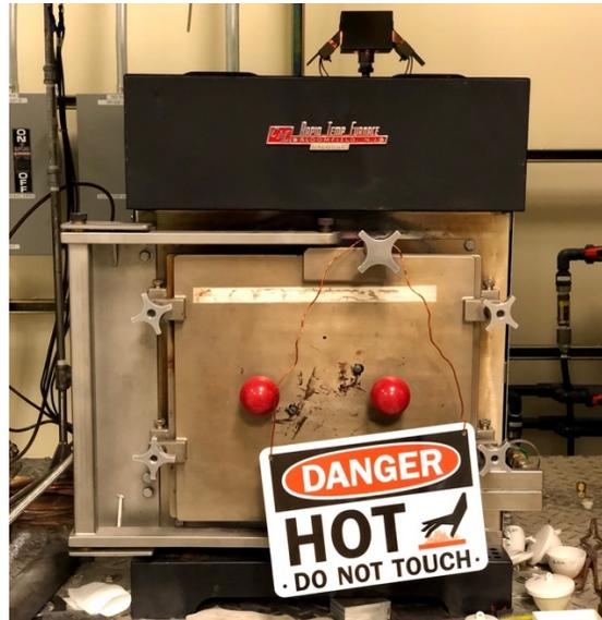
Figure 35: Rapid Temp Furnace by CM Inc. used for homogenizing and heat treatment
