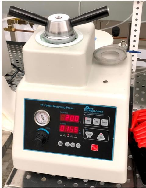
Figure 42: TP-7001B Mounting Press by Pace Technologies
