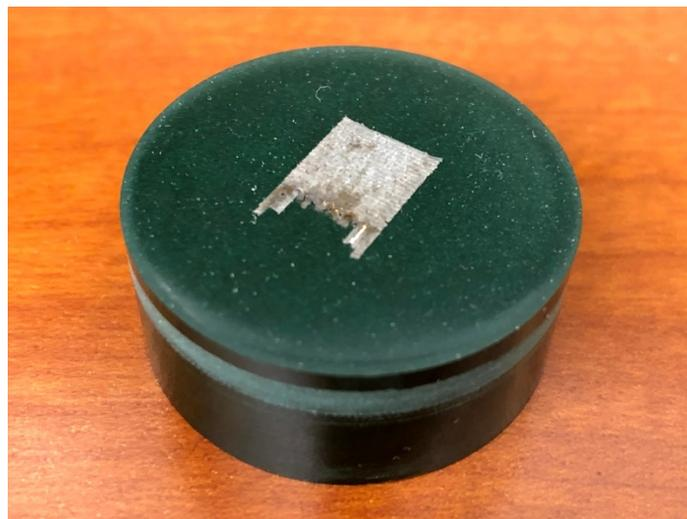
Figure 43: Mounted SLMed specimen ready for metallography
