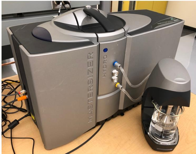
Figure 30: Malvern Mastersizer3000E particle size distribution analyzer
