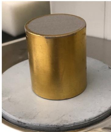
Figure 33: Levelled H13 powder in the collection cup
