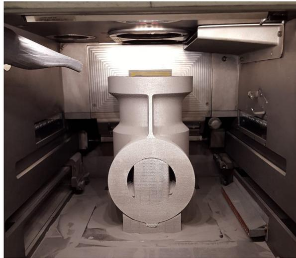
Figure 12: A titanium alloy aerospace component in an SLM chamber upon completion [36]
