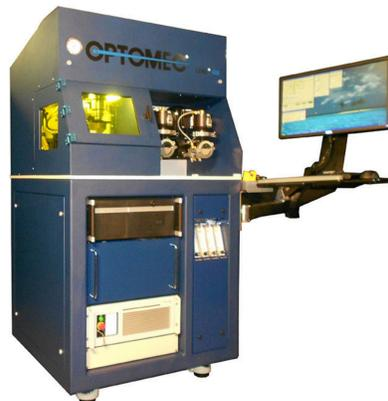
Figure 9: The Optomec LENS® 450 system [31]
