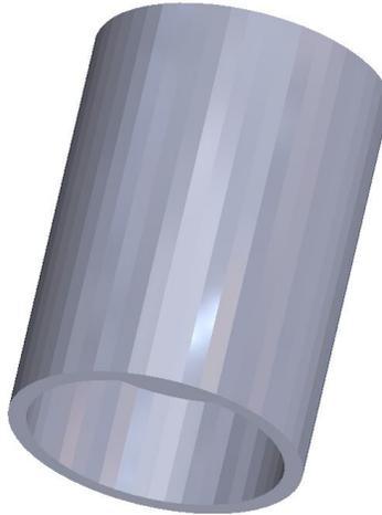
Figure 36: SLMed specimen with orientation where the Z-axis of the machine points upward through the cylinder. The ring at the bottom provides additional support during the SLM process
