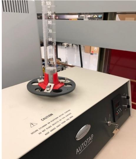
Figure 34: Tap density experimental setup using the Quantachrome Autotap used here
