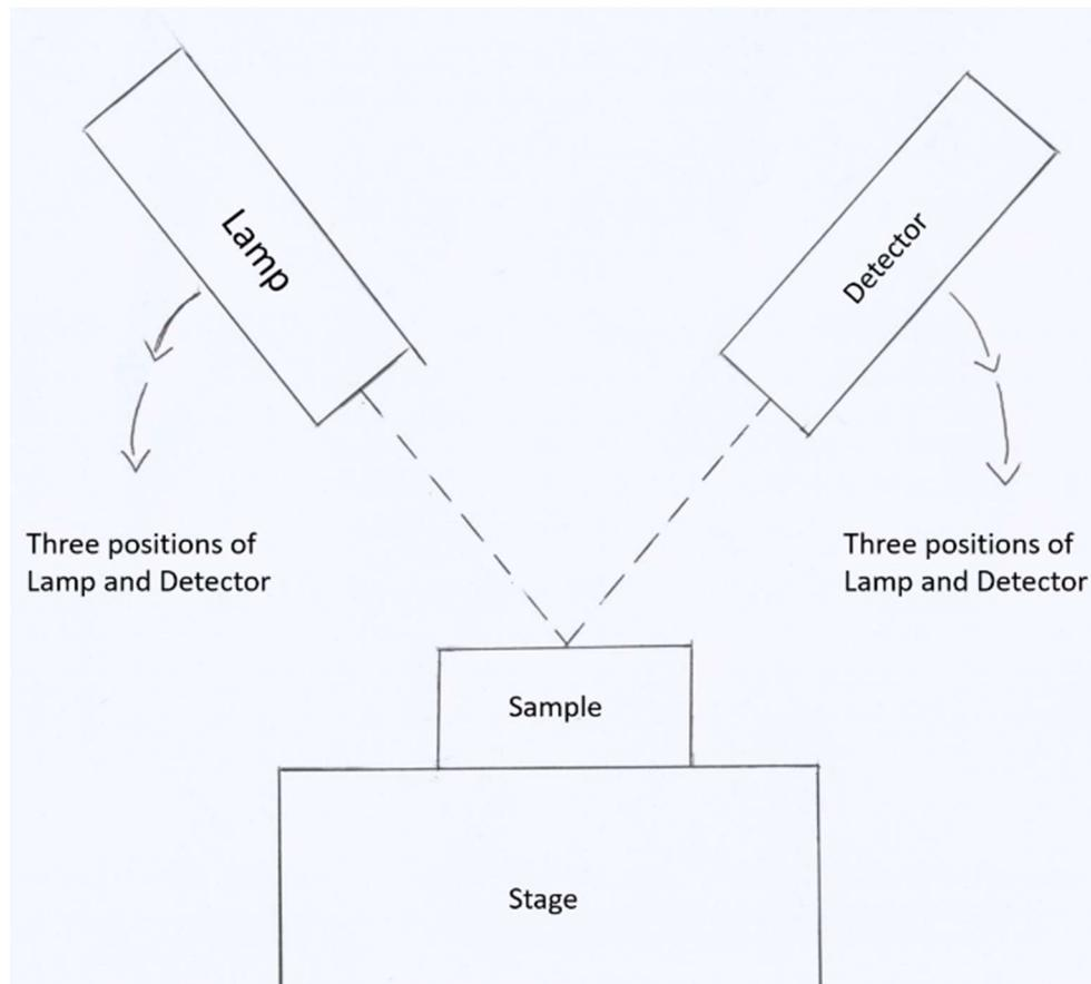
**Figure 1: Schematic of ellipsometer.** A laser is shined on your sample, and there are two reflections that are detected. One from the film itself, the second from the silicon disc the film is on. The ellipsometer has a program that detects the polarized light and the phase shift from the film and the silicon to determine the index of refraction as well as the thickness of the film.
