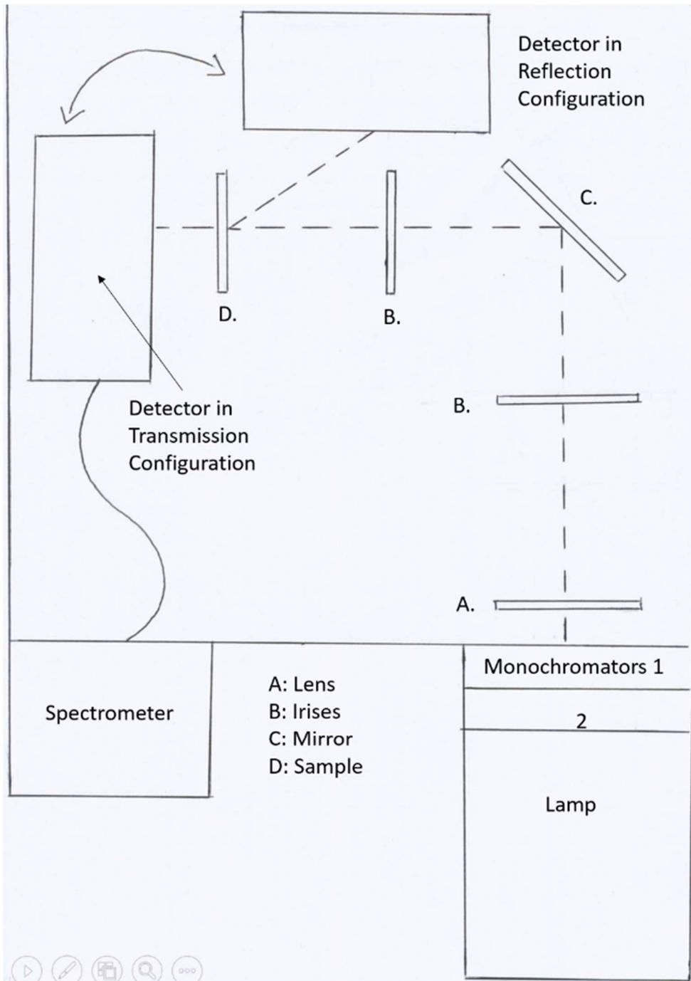
**Figure 3: Grating spectrometer schematic.** Everything but the lamp and monochromators are inside a box to block excess light to reduce noise. Lamp puts out white light which is filtered into a specific wavelength by the monochromators. The beam is directed through the sample and into the detector in either the transmission or reflection configuration.
