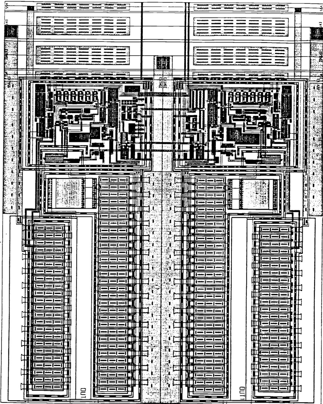
Figure 8. A layout for the differential line driver
