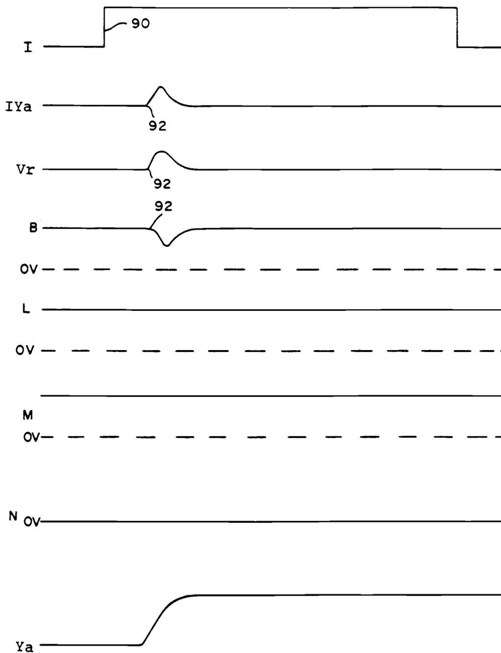
Figure 3. Signal waveforms at various terminals with the output non-shortened
