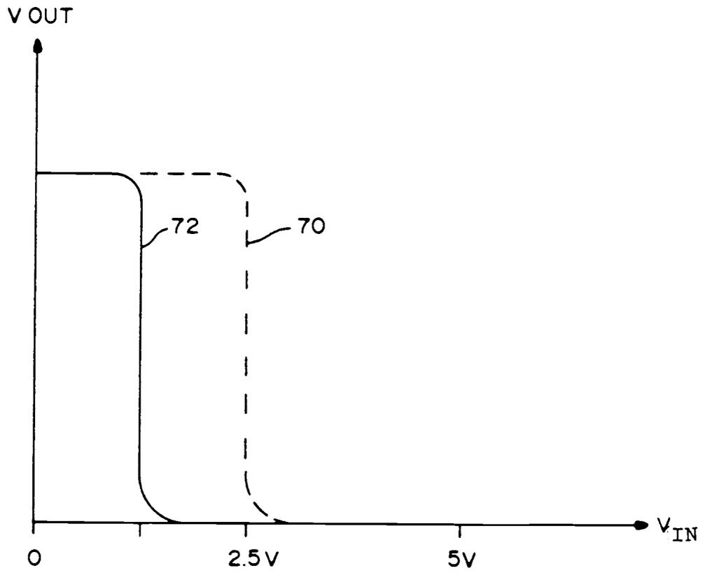
Figure 2. DC transfer curve of CMOS inverter
