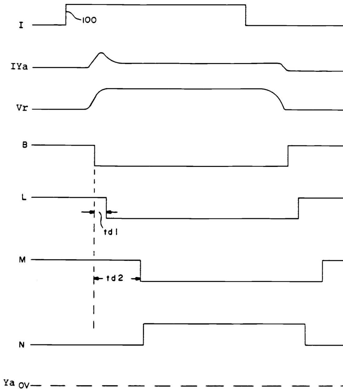
Figure 4. Signal waveforms at various terminals with the output shorted
