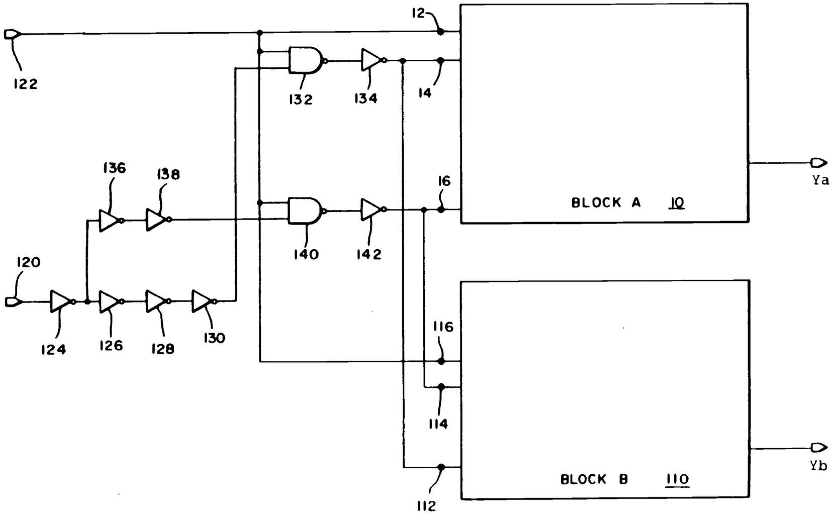
Figure 6. Schematic for complete differential line-driver system
