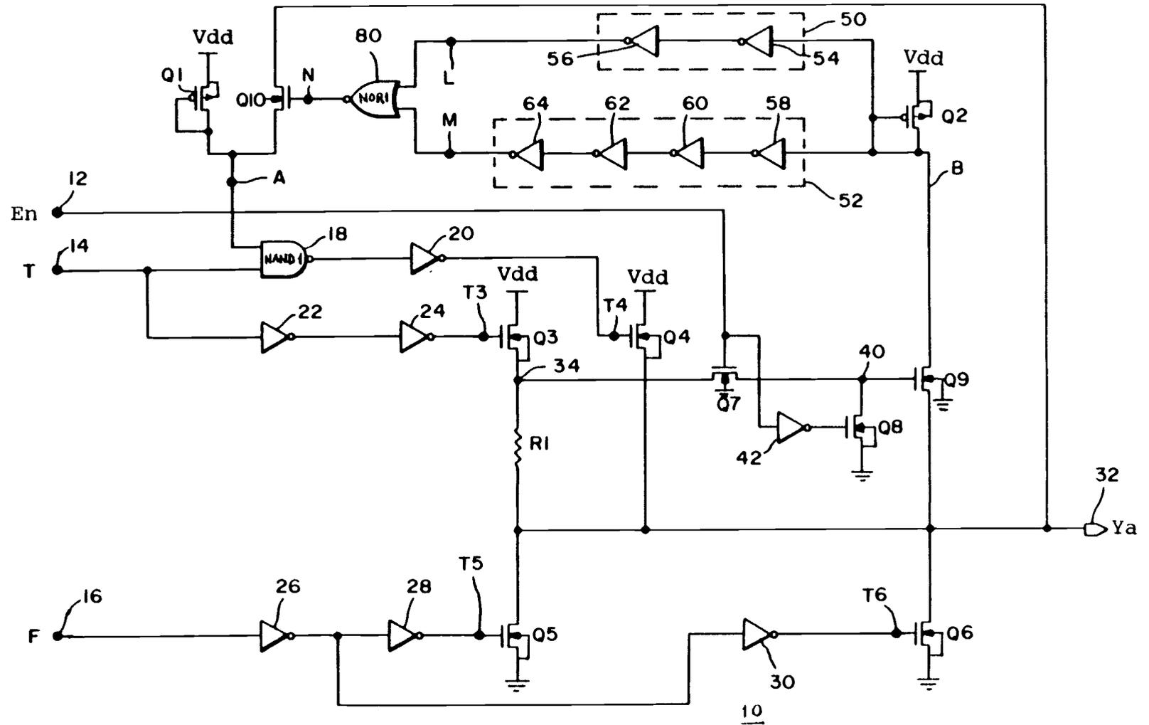
Figure 1. Schematic for line driver circuit
