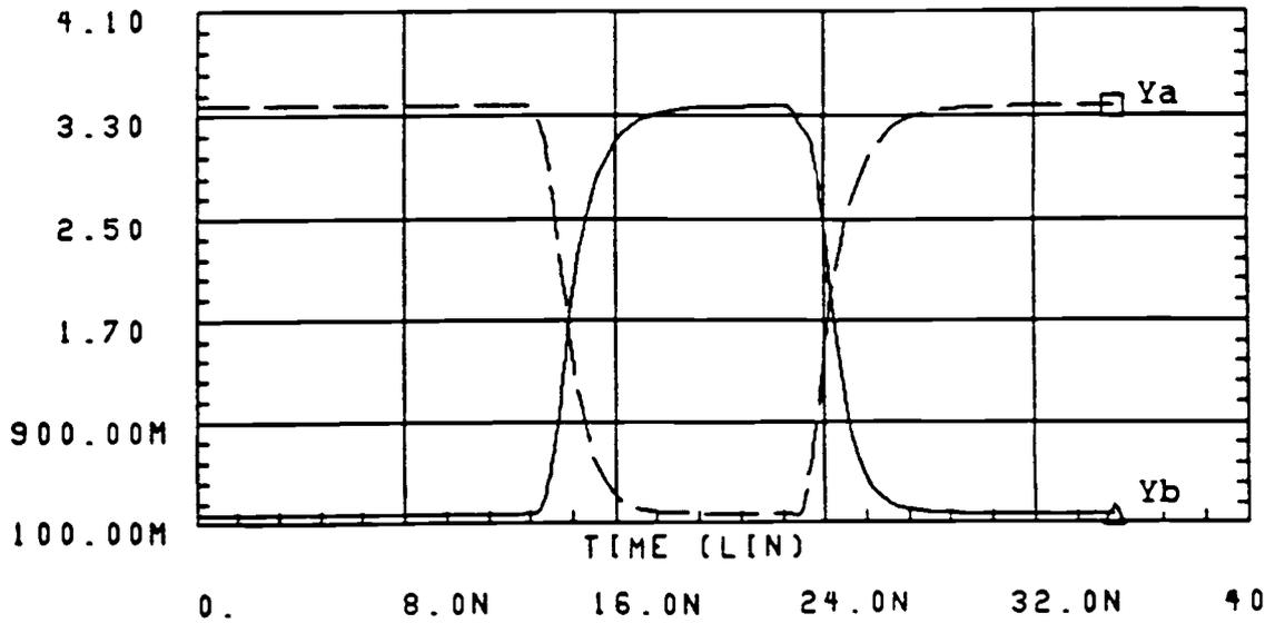
Figure 10. Output waveform of the line driver
