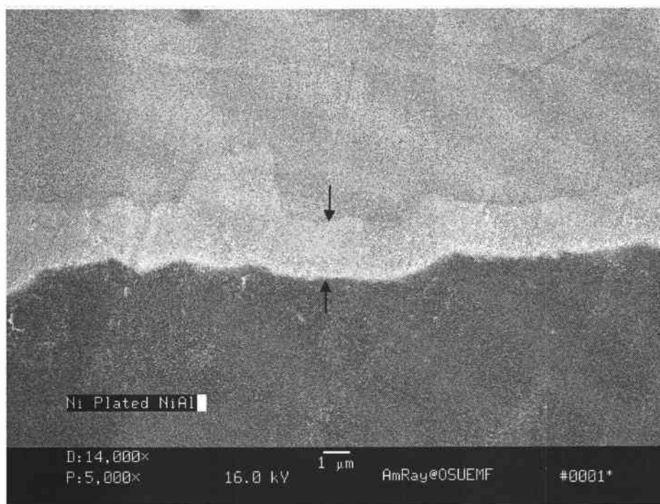
Figure 4.16. Scanning electron micrograph of Ni deposition on the side away from the anode after 100 minutes (5000X)
