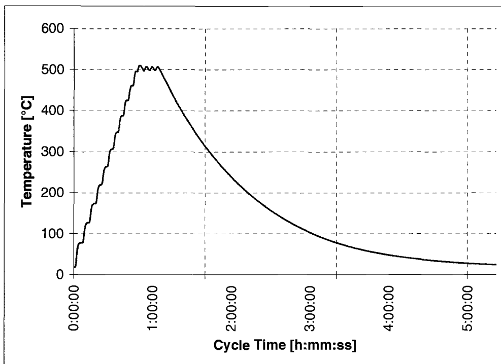
Figure 4.10. Temperature profile of NiAl tack bonding cycle
