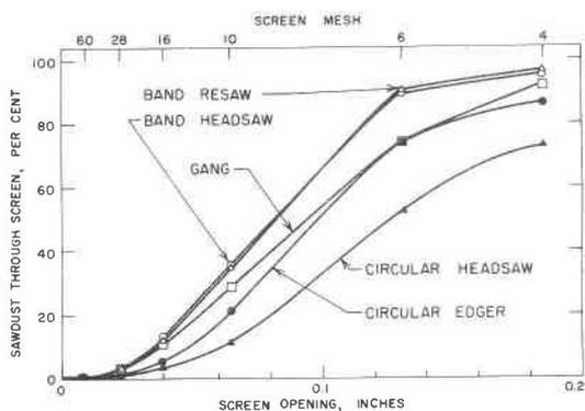
Figure 4. Average particle-size distribution of sawdust from a single saw of each type during a day at a Douglas-fir sawmill in the Willamette Valley.
