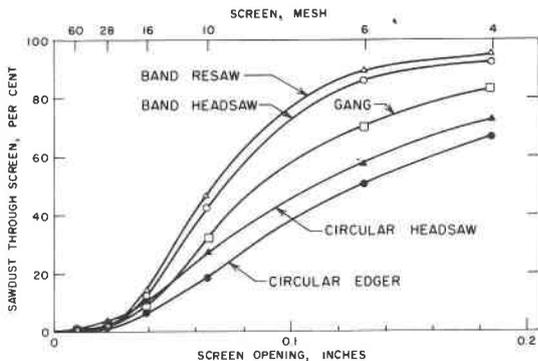
Figure 3. Frequency distribution, by weight, of sawdust particles from various Douglas-fir sawmills in the Willamette Valley.
