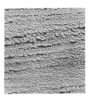
A successful maintenance program in which paint of soft type is used with long intervals between paintings. This house, which is next door to the one shown in the previous illustration, was erected in 1923, repainted in 1931, and has not been painted subsequently. The photograph was taken in 1936.
