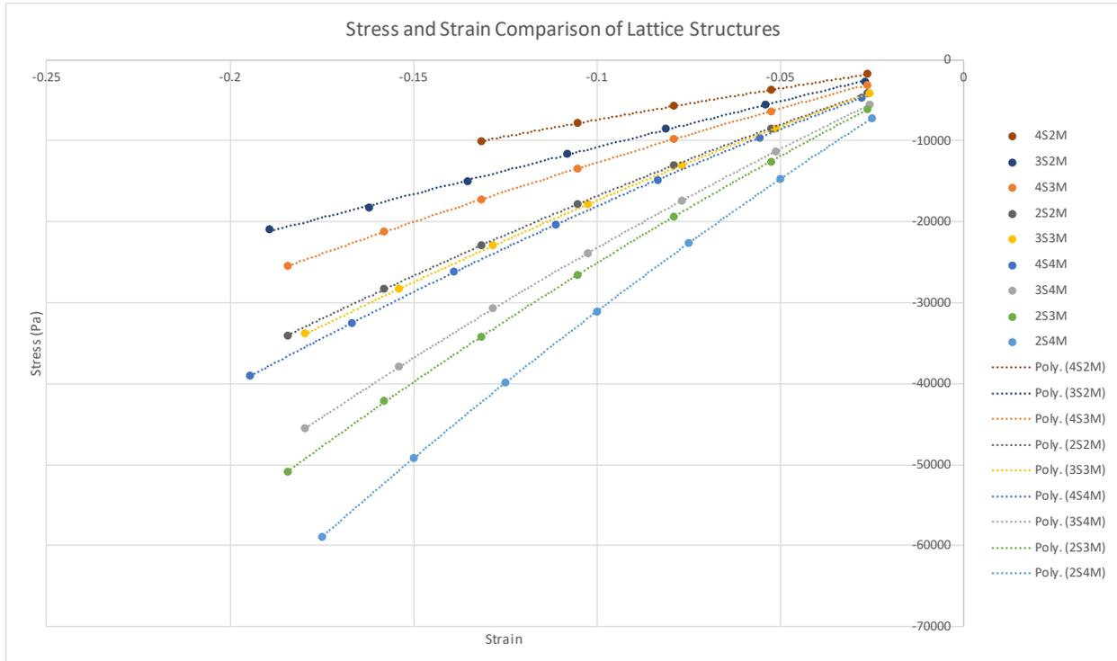
**Fig 9.** Comparison of the nine different lattice cubes with respect to strain and stress
