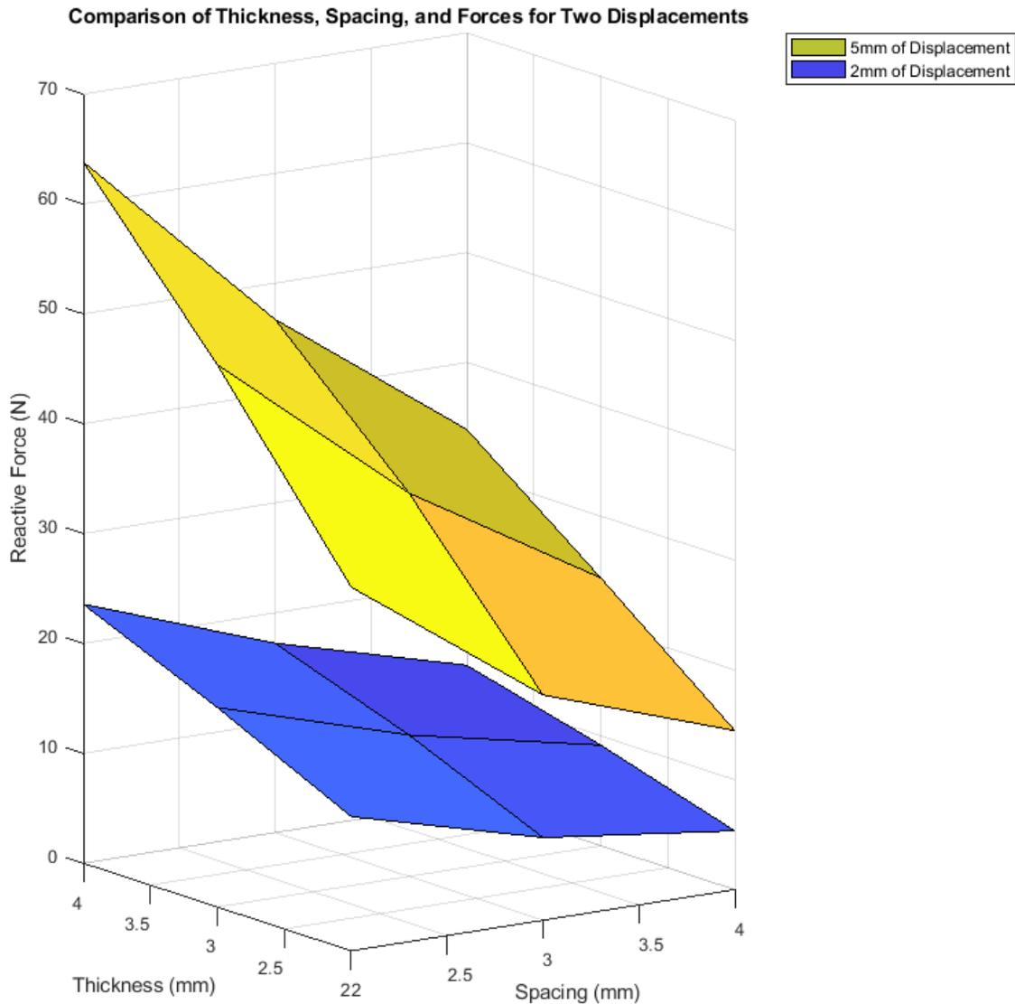
**Fig 8.** Surface plots of thickness and spacing with reactive force. Color gradient is based on the surface gradient
