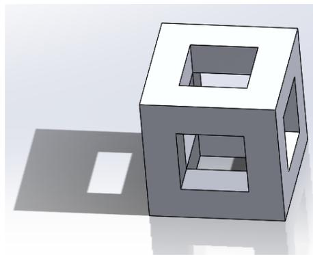
**Figure 3.** CAD model of the material property validation test article
