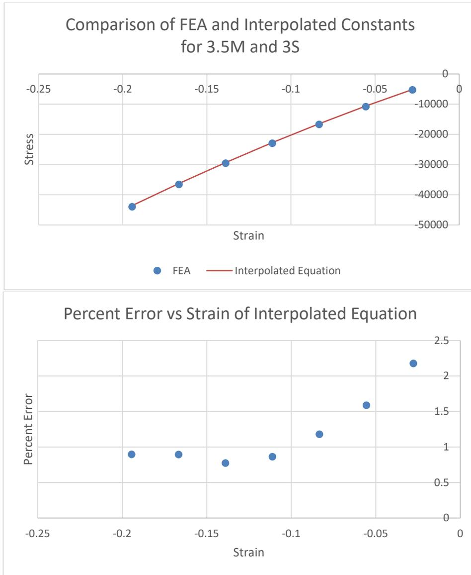
**Fig 11.** Plots comparing the interpolated equation and the FEA results of the 3S3.5M lattice cube
