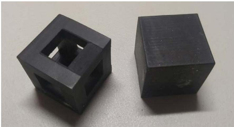
**Figure 2.** 3D printed test articles for (left) material property validation; and (right) material property measurement.
