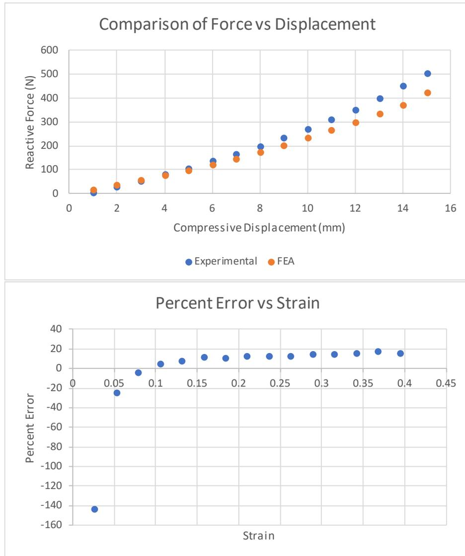
**Fig 6.** Plots comparing the solid cube experimental results and FEA results. As can be seen, after about 0.1 strain, the percent error is approximately 15%.
