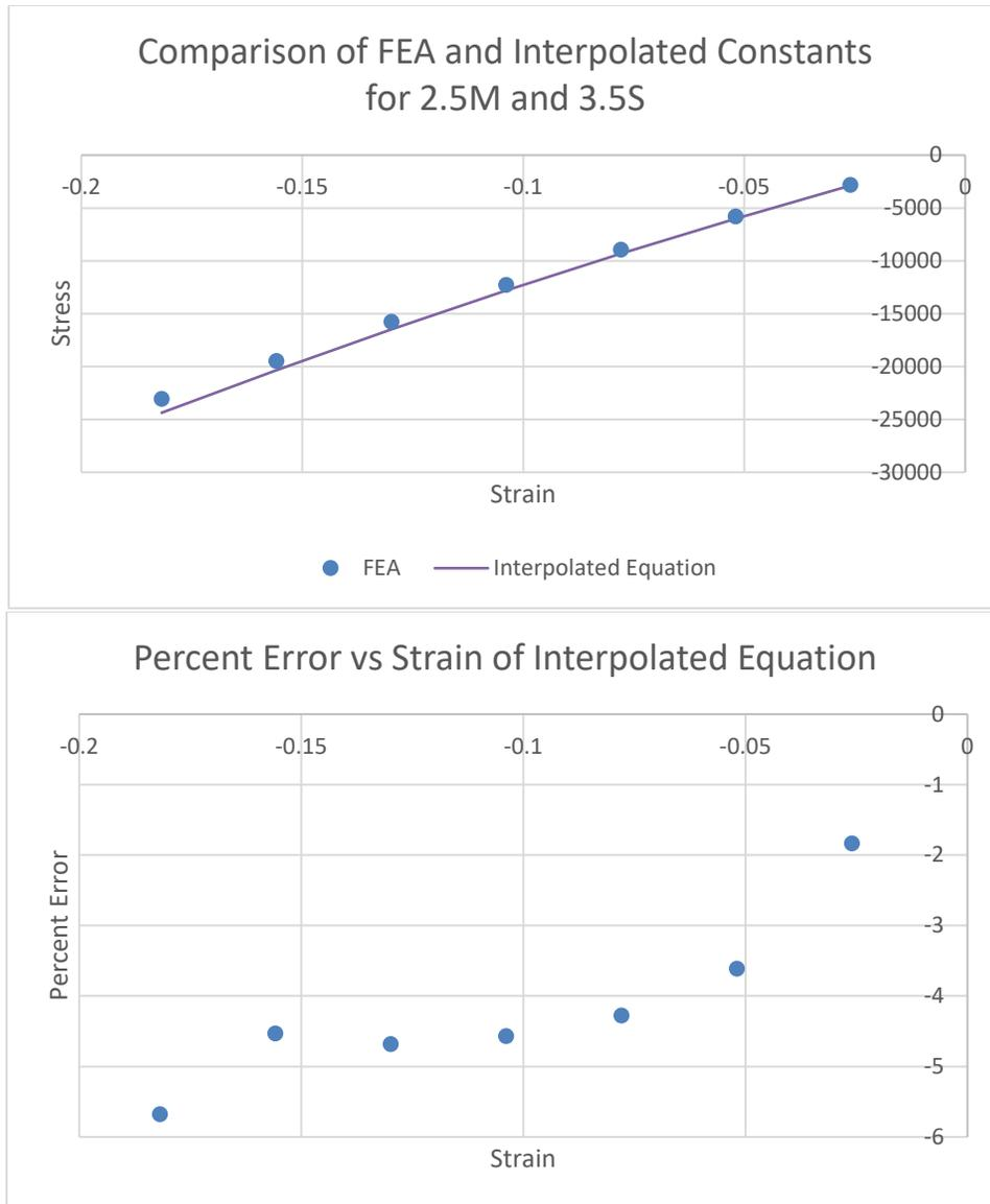
**Fig 12.** Plots comparing the interpolated equation and the FEA results of the 3.5S2.5M lattice cube
