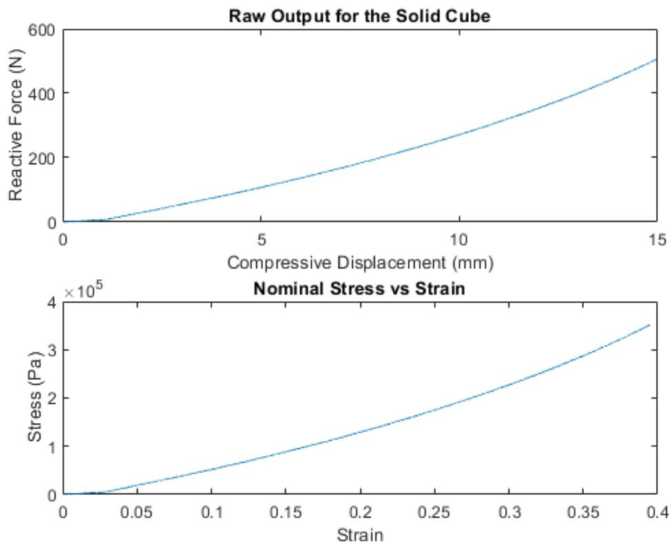
**Fig 5.** Plots showing the experimental data of reactive force versus compressive displacement of the solid cube as well as the calculated nominal stress and strain
