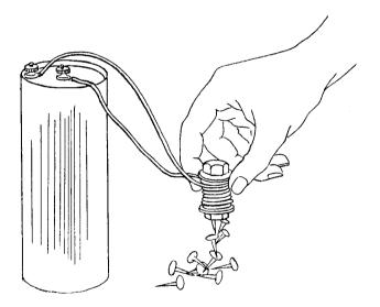
They are used in motors. Large electromagnets are used to pick up and move pieces of iron. The magnets are on large cranes. The iron is dropped when the electricity is turned off.
