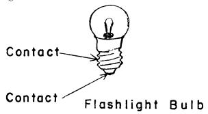
Batteries have two poles (contacts). If a conductor (wire) is provided electricity will flow from the plus pole to the minus pole.
